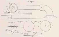
duction may be enhanced by making the reproducing stylus light, as by reducing its cross-section, but this reduces the volume of sound.
