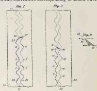
and also in a sound record having such diagonal arrangement of its complementary concavities and convexities.
