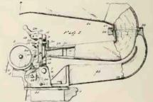
ported by the advancing carriage in approximately a horizontal plane. In case an amplifying horn was employed, such horn has been carried bodily on the front side of the reproducer carriage, to the end that the reproduced sounds might be directed by the horn toward the front of the instrument; or if a larger horn is employed, the same has been mounted upon a stand in front of the machine and connected to the top of the reproducer and on the front side of the carriage.
