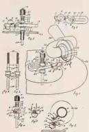
Figs. 4 and 5 are side views of spindle 20, the one transverse to the other. Fig. 6 is a transverse elevational view of Fig. Fig. 7 is a detail of the arm with the stop attachment thereon, and Fig. 8 a side view of the portion on the sound tube, in connection with the arm and its attachment, showing the
