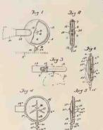
having a vibratory diaphragm held or confined in or on a suitable body, the edges being free or unconfined, as distinguished from an ordinary reproducer wherein the edge portion of the diaphragm is fixed or secured firmly to the body. Fig. 1 is a side
