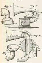
breaking at a point between the free ends thereof. said ball having means to be engaged by the parts of the amplifying horn, for the purpose of retaining them in their proper correlative positions, and in order to allow them to have universal movements
