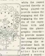
to provide a mechanism adapted to release a brake lever to allow the motor to run long enough to cause two records to be played and then actu-
