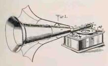
the diaphragm through concentric tubes so that the vibrations from the front of the diaphragm will so merge with the vibrations from the back of the diaphragm as to produce a large volume of tone of great distinctness, power and melody—to provide for removing the sound box from the record for replacing the needle or substituting the record—to counterbalance the sound box and accommodate its motion over the record that the grinding noise peculiar to most talking ma-
