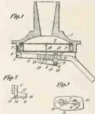
able of lateral movement, so that it will track the record groove properly; and it is also desirable that the stylus should be so connected to the diaphragm that the vertical movement of the stylus will be magnified, so as to produce an amplified
