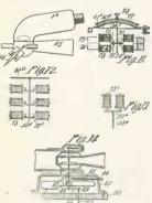
magnetically operated valve rod. Fig. 14 is a sectional elevation illustrating the use of the device in connection with a musical instrument having a sounding board, the sound waves being mechanicaltransmitted 1 ythrough the valves for the purpose of controlling the flow of the stream
