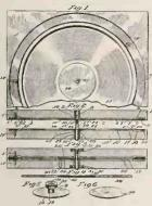
adapted to different kinds of presses now in use; to facilitate the removal of the finished record from the pressing device and to secure or fasten to the mold or pressing plate the matrices from which the sound records are pressed in the mold, and to provide other improvements.
