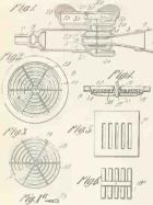
an enlarged scale Fig. 5 illustrates modified construction of seat. and Fig. 6 a modified construction of valve that may be employed. Fig. 7 is a sectional elevation illustrating a slightly modified construction that is adapted more especially for use as a secondary instrument and may be
