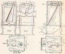
detail transverse vertical section of the means employed for supporting the pipe leading from the talking machine to the horn and the connection between the pipe and the horn. Fig. 4 is a vertical sectional view of a modified form of the
