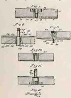
Fig. 2; Fig. 9 illustrates one manner of securing a label - depressing plate to either the upper or the lower pressing plate; Fig. 10, the plate so secured with the securing means removed; Fig. 11 shows a modified form of the lower plate and the label-depressing plate, and Fig. 12 is a plan view of
