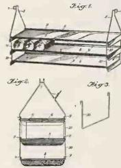
whereby the record wanted may be readily selected; also a construction by which the capacity of the rack may be increased as the selection of records is added to. In attaining these objects there is provided a pair of looped hangers having hooks for suspending them from a ceiling
