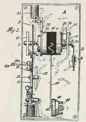
Patent Office Diagram of the Keen Lock, showing how the Electric Needle moves over the cylinder, Recording the Voice and Opening the Lock when the same Words and Tones are Repeated
