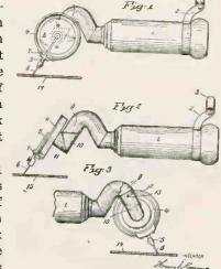
of the latter, and Fig. 3 is a sectional elevation of the sound-box and a portion of the tone-arm.
