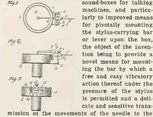
sound-boxes for talking machines, and particularly to improved means for pivotally mounting the stylus-carrying bar or lever upon the box, the object of the invention being to provide a novel means for mounting the bar by which a free and easy vibratory action thereof under the pressure of the stylus is permitted and a delicate and sensitive trans-
