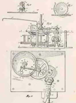
shown in Fig. 4. Fig. 8 is an elevation of the mechanism shown in Fig. 4, viewed from the right side thereof. Fig. 9 is an elevation, partly in vertical section along the line jz, of a detail of the mechanism shown in Fig. 8. Fig. 10 is a plan view of that part of the mechanism shown in Fig. 8 which is below the line lz.
