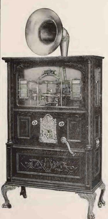
THIS instrument is equipped with twenty-four 10-inch flat records, from which a selection can be made, and both needle and record are changed automatically with one turn of the handle.
