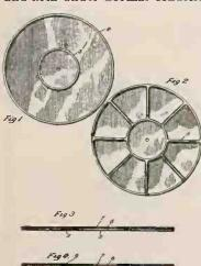
The material usually employed for making these records has been in the form of flat sheets and have been of uniform thickness throughout the entire extent of the disc, with the possible exception of the central portion where the label has been impressed or countersunk into the
