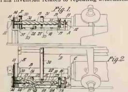
for phonographs, and its principal object is to provide a device of simple construction which may be readily attached to existing phonographs
