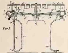
machines for revolving rotatable, cylindrical shells or other suitable holders, carrying molds, of the kind in which records or the blanks or cylinders for same for phonographs, graphophones and the like are made by pouring into them molten wax, or any other suitable material of which records or blanks may be made.
