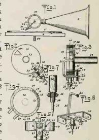
mitting vibrations from the needle to the diaphragm; Fig. 4 is a front elevation of the diaphragm box partly broken away; Fig. 5 is an edge view of the diaphragm showing means for adjusting the vibrator, which is pivotally mounted upon the diaphragm box; and Fig. 6 is a perspective of the vibrator and its accompanying mechanism for carrying the needle.
