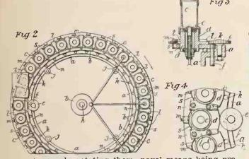
taneously rotating them, novel means being provided for successively moving the molds out of operative relation with the rotating means whereby the molds successively cease rotation in order that the product may be removed.
