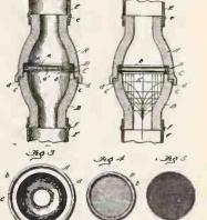
This invention, stated in general terms, consists of a device interposed in the passage of the produced and reproduced sound waves of such a character that the inharmonious produced sound waves are segregated or destroyed without interference with the reproduced sound waves whereby the reproduced sound waves are obtained with clearness and accuracy, and consists of a combination of elements and devices as hereinafter clearly set forth, reference being had to the accompanying drawing.
