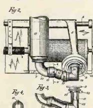
chine, Fig. 2 is a top view of a portion of the same, Fig. 3 is a sectional detail view showing the tubular connection between the tone arm and reproducer, and Fig. 4 is a sectional detail view on line 4—4 of Fig. 3.
