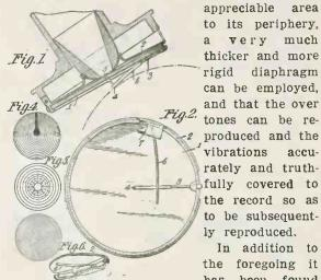
to its periphery, a very much thicker and more rigid diaphragm can be employed, and that the over tones can be reproduced and the vibrations accurately and truthfully covered to the record so as to be subsequently reproduced.
