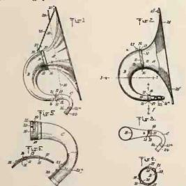
struct the horn in three separable parts, namely, a bell section, a body section, and a tip section, in order that the horn may be stored in a minimum of space.
