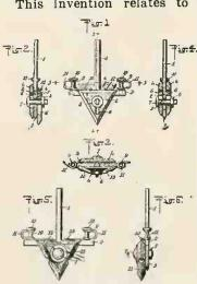
and has for its object to provide a stylus which can be adjusted in numerous different ways so that it will always have a good point to trace the record, thereby actuating the diaphragm in such a manner that the sound waves produced will be and the even sounds harmoni-
