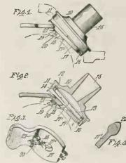
waves or beats affect the diaphragm on truly concentric lines starting from the precise center of the diaphragm, and the stylus receives an accurate vibration in accordance with the impressions the record, and conveys them with the least resistance and a
