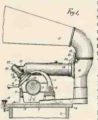
reproducer movable across the same, and a tone pivotally arm mounted at one end and having its free end connected to the reproducer. The object of the invention is to effect certain improvements in the construction of machines of this type with respect particularly to the devices for sup-
