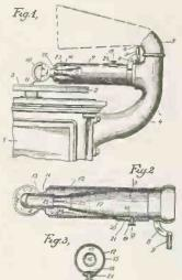
in the motor box of the machine, and which connects with an amplifying horn, the sound-modifying devices being located within this tubular tone arm and adjustable from outside the same for the purpose of effecting the desired modification in sound.
