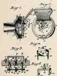
stylus lever for actuating the same, and the means employed for allowing the stylus lever to turn or rock in a direction approximately parallel to the diaphragm; Fig. 2 is a rear elevation of the reproducer, showing how the stylus lever is mounted upon the rocking disc by
