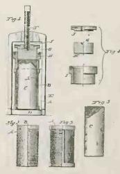
employed to force the outer face of the phonogram blank into contact with the matrix.
