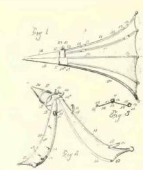
means for holding these separable sections when they are assembled to form the horn, and a still further object is to provide a means on the smaller end of the horn for holding all parts together, so that the small and large ends are rigidly and secnrely connected.
