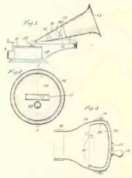
the purpose of softening the tone and removing the nnpleasant metallic timbre that is frequently present. In the accompanying drawings, forming a part of this specification, Fig. 1 is a side view of a phonograph or graphophone with a portion of the horn broken away to show the modifier device in place therein. Fig. 2 is a top plan view of the modifier, and Fig. 3 is a sectional view on the line 3 3 of Fig. 2.
