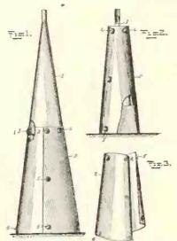
a removable outer section which may be wrapped about the small end of the horn in order that the whole may be packed in a small compass.
