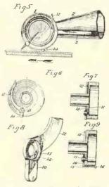
the same sound box shown in Fig. 1. Figs. 3 and 4 are detailed views of the means for retaining the safety device in its operative position. Fig. 5 is a front elevation of a sound box embodying another form of the invention; Fig. 6, a rear elevation thereof; Fig. 7, a transverse sectional view; Fig. 8, a view of the safety device detached from the sound box; Fig. 9, a view showing a modified form of the safety device or guard, and Figs. 10 and 11 views showing another form of safety device.
