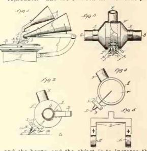
and the horns, and the object is to increase the volume of sound and improve the tone of the instrument. Fig. 1 is a side view of the gramophone, showing the reproducers, connections and horns in position supported by the bracket and
