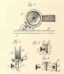
and enlarged; and Fig. 4 shows the parts of the improved clamp separated and ready to be assembled, the removable jaw being in section and the other parts in elevation.
