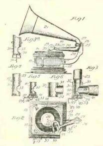
mercial type of phonograph-horn, whereby great accuracy of regulation of the volume of sound-waves passing through the horn is obtained.
