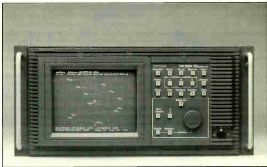
The Tektronix VM700A combines waveform and vectorscope functions with a noise measurement set and data logger.
