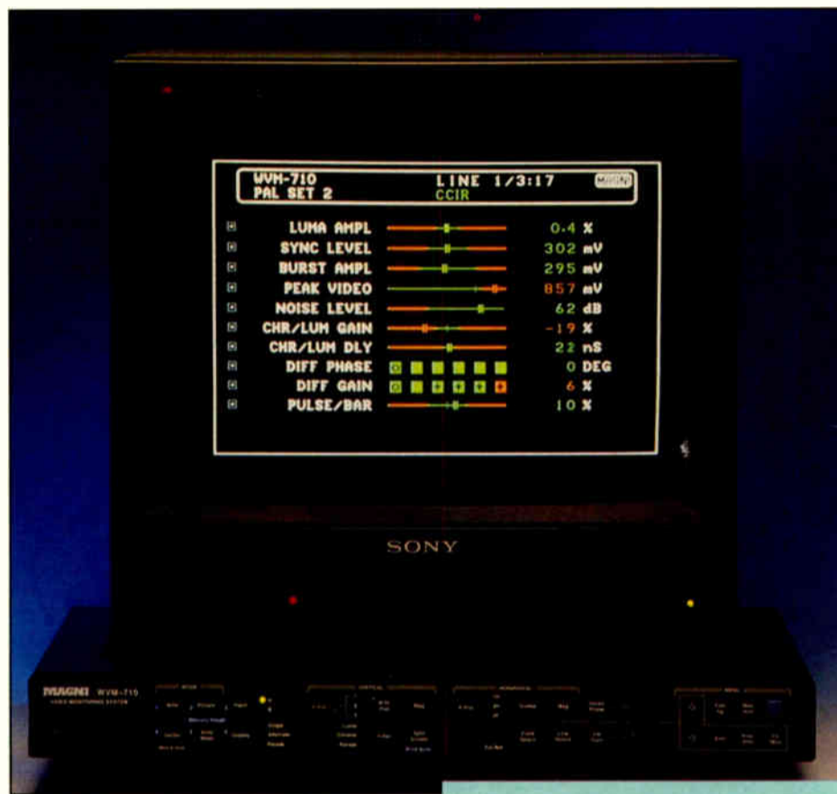
The Magni WVM-710 stores six vectorscope readings for later recall.
