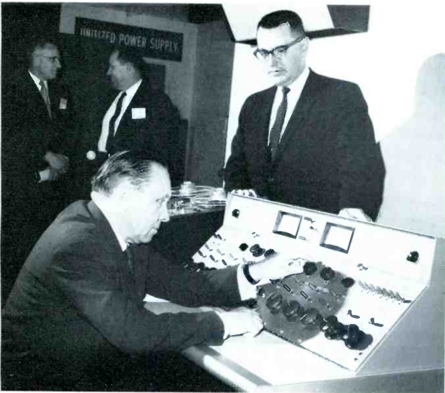
AT THE CONTROLS of the RCA transistorised consolette, the Editor of International TV Technical Review and his team are shown the functioning of this BC-7 for dual-channel AM/TV and FM stereo by RCA's Mr. C. D. Sullivan. This consolette uses interchangeable plug-in modules, and has colour-coded controls functionally arranged.
