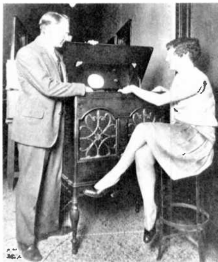
A 1929 Westinghouse tv set, above, being demonstrated by famed tv inventor Vladimir Zworykin, who later worked for RCA. (He invented the iconoscope.) Picture is projected from a mirror. In late 40s, "Uncle Milty" Berle, performing in outrageous costumes, dominated video and won the name, "Mr. Television."
