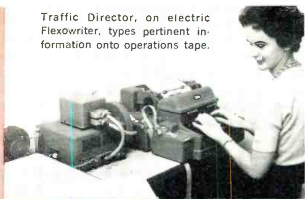
Punched tape is fed into "tape readers" which first stores information in master control data storage and processing area, and then actuates electronically timed and coded equipment into any switching operation desired.
