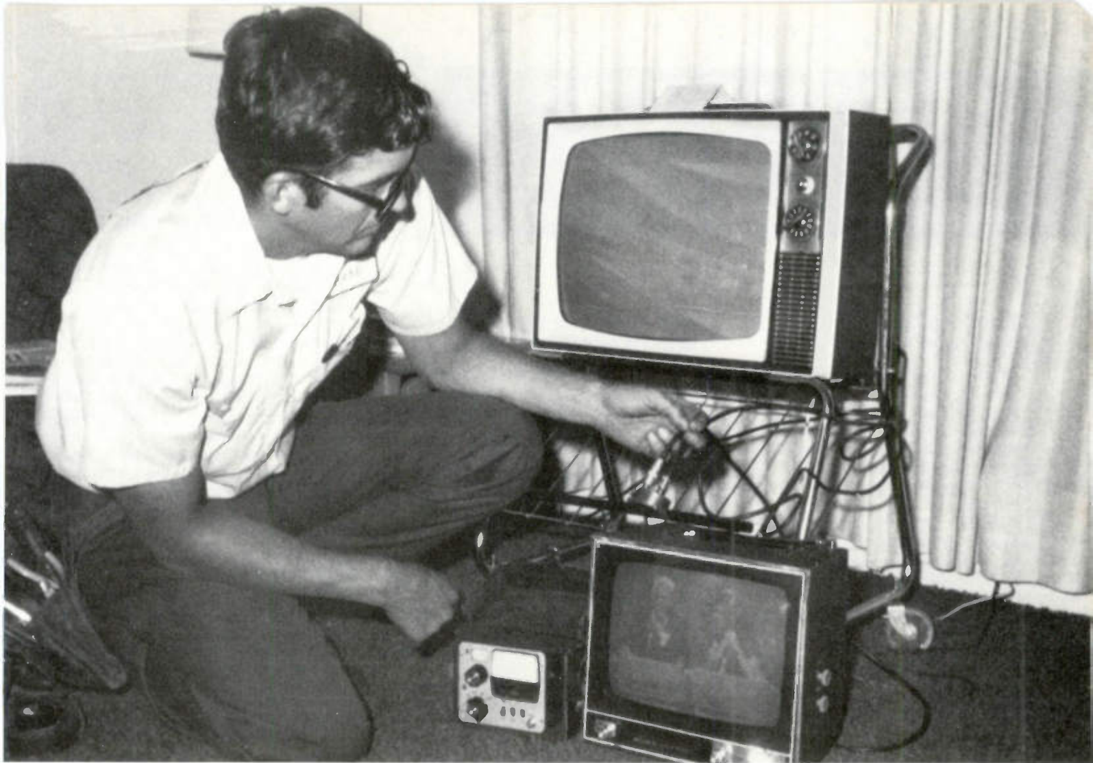
Author Brad Prowse uses a splitter to run both the test set and the customer's set at the same time, to best illustrate to the customer that the trouble is located in his set. Photo courtesy Gold Hills Cable TV, division of Nation Wide Cablevision.
