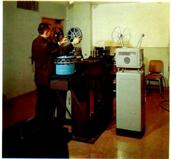
Film chain and slide unit are part of many local origination operations. Shown here is the equipment used in the showcase cablecasting studios of Cleveland Area Television's Lakewood, Ohio system.
