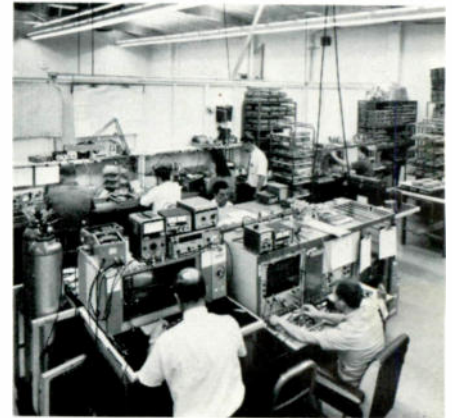
The last mile — test and alignment. All amplifiers are tested both before and after they are installed in housings.
