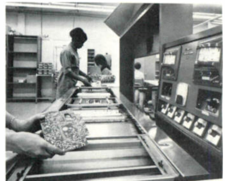
A flow-solder machine attaches components to an amplifier circuit module.
