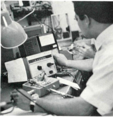
A staff engineer uses a VHF oscillator and precision RF volt meter to check pre-equalization of distribution amplifier outputs.
