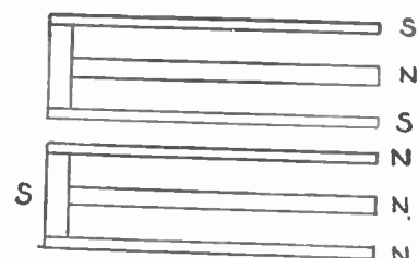
Fig. 2. The diagrams show the poles developed in the mysterious magnet by exciting the coils in different ways. In one case we get north and south poles at one end; in the other case they are all north at one end, with a south pole at the other.
