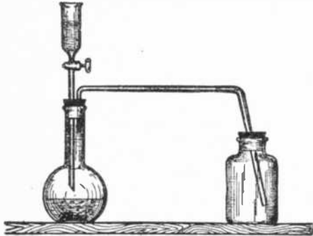
Collecting sulphurous oxide by upward displacement of air. The gas is a little more than twice as heavy as air and therefore can be thus collected. The funnel tube need not dip into the liquid because of the stop-cock.
