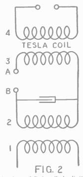
Another form of Tesls coil circuit employ-ing only one condenser. The operation of this circuit is very similar to that of the hook-up shown in Fig. 1.
