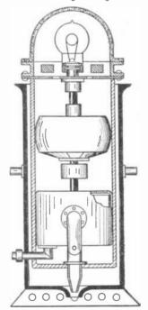
This very compact lighting outfit contains a small hydraulic turbine directly connected to the shaft of a small electric generator which supplies power to the incandescent bulb. The turbine is connected to a faucet. Patent No. 1,528,754 issued to M. Bresson, Douai, France.
