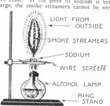
Interesting experiment with burning sodium; the experimenter must be very careful, however, to keep face and hands away from the melting metal.
