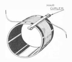
Fig. 3. Indicating a cylindrical form for winding solenoid coil. A hair curler, as shown in the illustration, may be used to fasten the wire temporarily so that it will not unroll.
