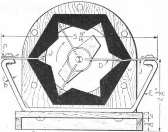
The top and side views of the minature electric motor. The interaction between the peculiarly shaped soft iron stator and the rotor armature causes the latter to rotate. It will be noted that in place of the usual commutator three radial spring strips are employed.
