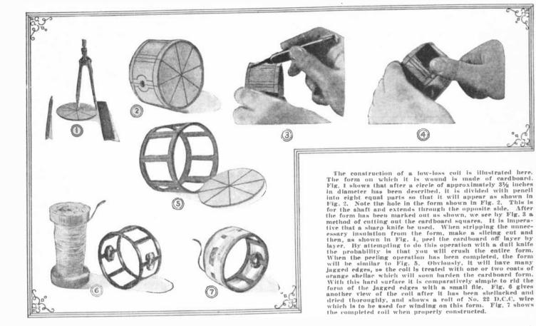
N the making of the ever-popular low loss coil, many experimenters overlook completely the element of mechanical strength which is necessary in order to keep
