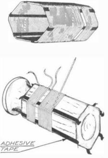
Fig. 2. The two drawings shown above indicate how a pickle-bottle coll may be used as a form for winding a good low loss coll. Six pieces of adhesive tape are placed gummed side up, and the wire wound over the adhesive... Not only does the adhesive reinforce the coll by holding each individual wire, but losses through absorption are not as high as when using the usual cylinder wound coil.
