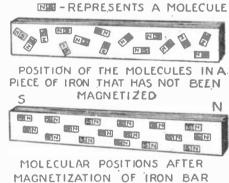
According to one magnetic theory each molecule is a small magnet. When a bar of iron is unmagnetized, these small unit magnets are disposed in a haphazard manner. When, however, the body is magnetized, they assume a position with all north poles facing in one direction. These two conditions are illustrated diagramatically above.
