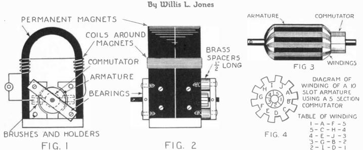
Figs. 1 and 2 show the end view and side view of the generator to be operated by the motor. Figs. 3 and 4 show the general disposition of the armature with a very clear table for the winding.
