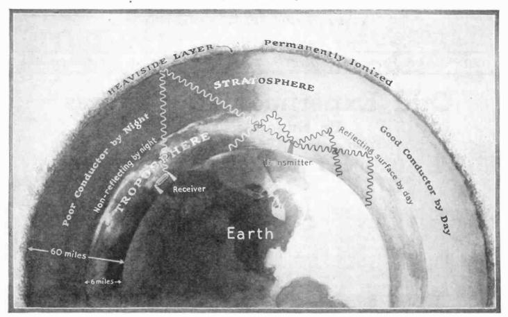
Fig. 1. A cross-section of the atmosphere according to the Heaviside theory of electromagnetic propagation. Note the transmitter in the daylight region sends out waves which are on the daylight side reflected at the stratosphere and so traverse but short distances. However, a wave crossing the day and night line before reaching the stratosphere will continue until it is reflected from the Heaviside layer and so will traverse much greater distances on the night side than on the day side.
