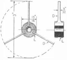
The three contact springs of the rotor and the hub or boss to which they are attached.
