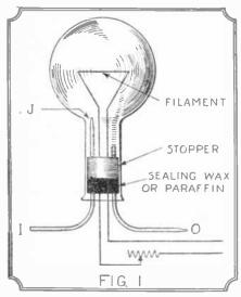
Decomposing a hydrocarbon gas by an ignited filament. Chemical decomposition is the result, with deposition of carbon. The hydrocarbon gas enters and the gas which leaves while not pure hydrogen is considerably poorer in carbon.
