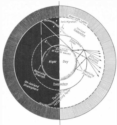
I Fig. 2. Diagram illustrates various forms of propagating radio waves. Reflection from the stratosphere involves great loss of energy through diffused radiation. Similarly waves propagated through the earth lose much of their energy upon reflection through the interior surface.
