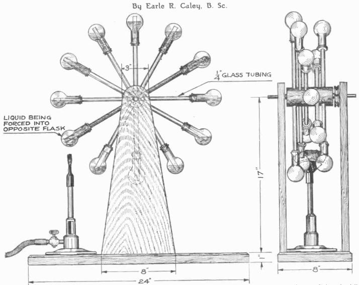
This ingenious motor operates by the fluid being forced over to one side of the axle by the heat of a Bunsen burner. It is a chemist's motor, being made up of chemical supplies. It is well to have a fan tip for the burner if the tubes are arranged as shown.
