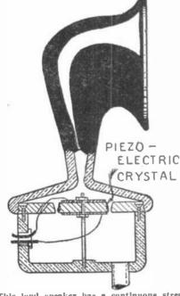
This loud speaker has a continuous stream of air passing through small orifices whose size is controlled by the piezoelectric crystals in accord with the variations in the electric current. Patent No. 1,526,319 issued to L. W. Chubb, Edgewood. Pa.
