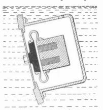
This is another form of vibrating apparatus producing sound waves under water for sound-ing and signaling purposes. The device is a modified form of telephone receiver. Patent No. 1,528,414 insued to A. du Bois-Raymond, Plon, Germany.
