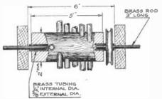
The shaft and central mounting of the chemical motor are shown above partly in section. It is essential to avoid friction and have good hearings for the shaft shown extending to the right and left.
