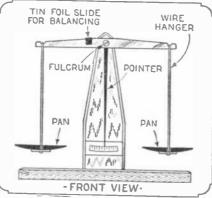
Front view of a balance which can be used by the amateur chemical experimenter and which weighs with sufficient accuracy for every-day work.
