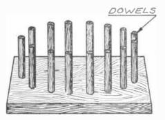
Fig. 1. Fifteen dowels are arranged in a a circle  $3\frac{1}{2}$  inches in diameter on a square baseboard 5 x 5 inches. To wind the basketweave coil, for which this form is used, the wire is wound in and out of the pegs, in an alternate manner. The pegs are approximately one-quarter lnch in diameter.
