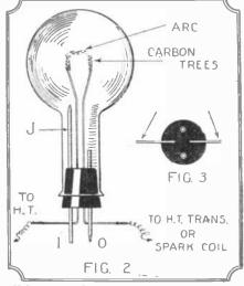
Using a spark or arc discharge for effecting the decomposition as described. A spark coil or high potential transformer can be used. A sort of bridge of carbon from electrode to electrode is produced.
