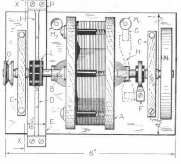
the holes must be worked out at exact right angles to the face of the wood.
