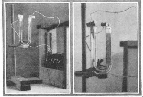
In a short while the snode or positive connection to the battery will be surrounded by a red solution showing that this leg of the U tube has an acid reaction. When potassium permanganate is placed in such a U tube and a current is passed through, a migration of ions also takes place, the colored ions traveling to the positive electrode which leaves the other leg of the tube colorless.
