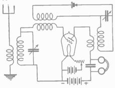
Fig. 1. A one-tube reflex receiver using a crystal for detector. Volume is good and distance greatly increased by the addition of the reflex system.
