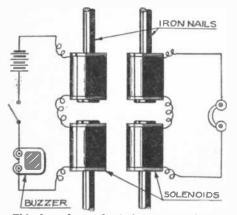
This is a form of wireless communication, though of course effective only over a distance of a few inches, Pulsating current in the coils on the left induces an c.m.f. in those on the right.
