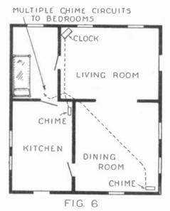
A master chine clock may be made to play a set of chimes, a different time each quarter or half hour, as the case may be, placing the different sets of electrically rung chimes in various rooms of the house. The respective ringers are connected in parallel with the main switch wires coming from the clock.
