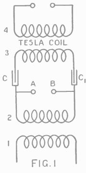
The diagram shows one type of connection for the Tesla coil. (1, 2) is a step-up trans-former. C and C<sub>1</sub> are condensers of equal capacity.
