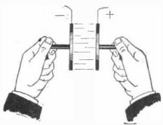
Alessandro Volta discovered that when two discs of unlike conducting materials are brought in contact and then suddenly separated, they will be charged to opposite polarities and in some instances give potential differences of over one volt.
