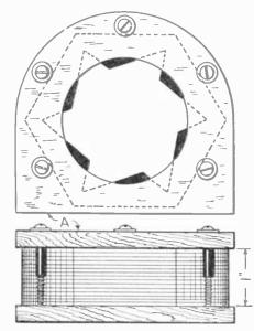
Assembly of the soft iron stator. The laminations are clamped between two wooden boards by means of large wood screws.
