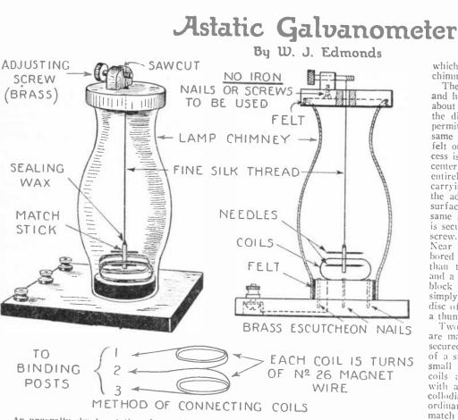
An unusually simple astatic galvanometer may be constructed as shown above. An astatic galvanometer has an advantage over the ordinary galvanometer in that it is not influenced by the earth's magnetic field. Two magnetized needles are employed disposed in opposition to each other so that the turning forces on the two needles due to the earth's field are neutralized.
