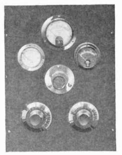
Fig. 1. Front view of the short-wave transmitter. The two lower dials are the condenser controls. The center knob is on the primary rheostat, while the two meters immediately above are the plate current and radiation meters. The top instrument is an A. C. voltmeter,
