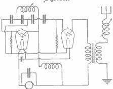
The inventor of this circuit claims that the The inventor of this circuit chains that the usual danger of overloading the tube when the radiating system is tuned to the oscillator, is eliminated. Patent No. 1,526,311 issued to M. C. Batsel, Wilkinsburg, Pa.
