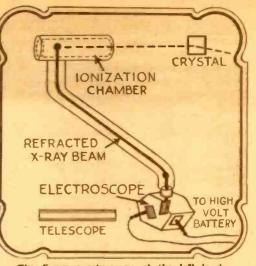
The X-ray spectroscope at the left is designed to study the arrangement of atoms in a crystal. As shown above, the X-ray is refracted by the crystal, and enters the ionization ehamber, producing an electrical charge which affects a gold leaf electroscope.
