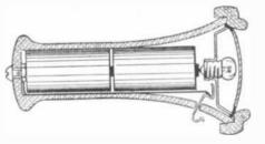
This very unusual flashligh is ingeniously constructed out of a discarded Bell telephone receiver case and a few old brass parts.
