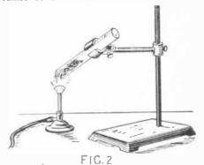
Igniting the dull tinted precipitate of tin salphide, having first mixed it with flowers of sulphur and ammonium chloride in the proportions given. The temperature is kept rather low and shortly after the fumes cease, the tube is allowed to cool, and will contain a quantity of beautiful golden yellow scales.
