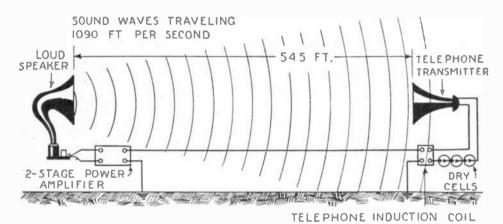
With a steady battery supply and other correct conditions, the above become a perpetual radio which will furnish no end of fun. A distance of at least 500 feet should separate the two instruments.
