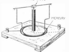
The simplest possible production of the rotating conductor in a magnetic field, following out Faraday's well known work.
