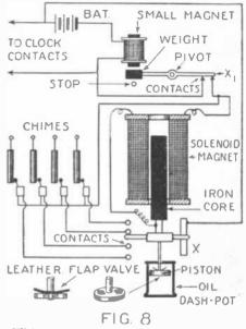
With a set of revolving drum switches controlled by a motor, the experimenter will find it very interesting perhaps to try out magnetic solenoid switches, as shown in Fig. 8 above. Here the upward motion of the solenoid core is retarded by a dash pot, and the main circuit to the ringers is automatically opened as the core and contact arm descend; otherwise the ringers would play in reverse fashion.
