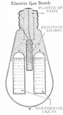
This device shaped, like the usual incandes-cent bulb, is exploded when a button conven-lently placed is pressed. In case of bank burglary, a clerk presses a button, setting off the bonb. This distracts the attention of the burglar and gives an opportunity to the clerk to duck behind the counter and apply his gas mask while the burglar is overcome by the in-canacitating gas. Patent No. 1,526,351 issued to R. D. Lawrence, Bellevue, Pa.
