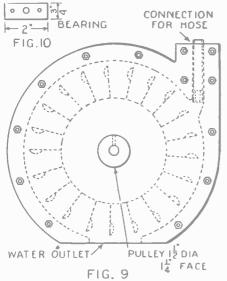
Side view of the hydro-motor with dotted profile of the gong and dippers, and the bear-ing for the shaft is shown in the upper cor-
