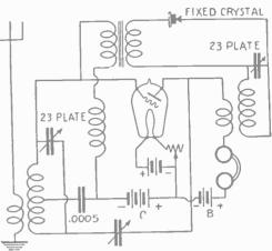
Fig. 3. Another one-tube reflex circuit. This circuit is very selective as well as being unusually sensitive. Both condensers are 23-plate (.0005 mfd.). In connection with a good aerial and ground system very good results may be obtained from any of these circuits. A hard tube is used in each circuit.
