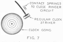
Where the hour is to be struck with the number of beats corresponding to the hour, the regular gong hummer or chapper on the clock may be caused to close a pair of contact springs, as shown above in Fig. 7; moving the gong so that the hummer cannot strike it, or the hammer may be bent. The contact springs come from an old radio or telephone jack.
