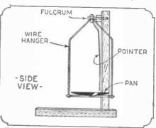
Side view of the balance; the hollow pans and long pointer are here shown clearly.
