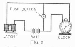
The diagram illustrates the circuit for the automatic operation of the electromagnetic window closing device. The usual arrangements can be used for closing the circuit with the alarm clock mechanism.
