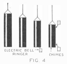
Brass pipe chinies hung from strings may be rung with electric bell ringers, placing the ringer in the position found by experiment to be best. Several, suggested positions for these ringers are shown above.
