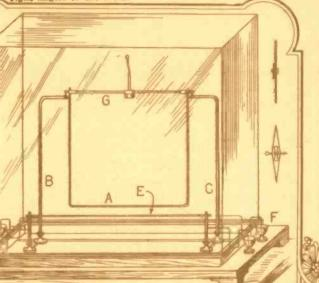
The famous French physicist Ampère, a contemporary of Ocrated, following up the latter's experiments, studied the interaction be twe en the magnetic fields of two paralled wires. The wires A and E can be made to carry current in the same or opposite directions. A mpère studied the repulsion and attraction between the two whres.
