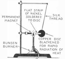
That magnetism is a molecular phenomena is demonstrated by the apparatus above. A nickel strip when cooled is attracted by a permanent magnet. When heated, however, the nickel loses all magnetism and is released by the magnet.
