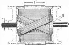
Assembly drawing of the rotor armsture and its winding. This armature has a shape peculiar to this motor and not usually found in dynamos.
