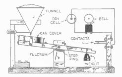
Here is an electric substitute for the hour glass. Sand falling from a funnel into a pan on one side of a beam scale accumulates there and when sufficient has fallen the beam is tipped and rings an alarm.
