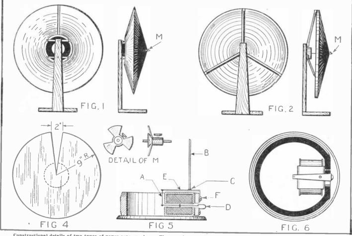
Constructional details of two types of paper cone speakers. The one shown at Fig. 1 has a closed back and the one at Fig. 2 an open back. A Bal-'win phone is used as the loud speaking unit.
