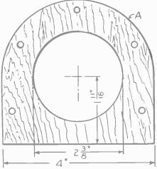
Detail drawing of the wooden frame supporting the soft iron stator of the motor. Large wood screws clamping the laminations are passed through the holes.
