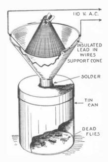
Human malice is here set against the innocent fly who when he alights on the conical coil of bared wire becomes electrocuted by bridging across a potential of 110 volts. An appropriate morgue is provided in the form of a tin can.
