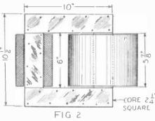
A dimension drawing of the core and the assembled transformer. The core is laminated and should be well bolted to prevent vibrations.
