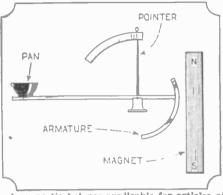
A magnetic balance applicable for articles of light weight such as letters; a really practicable form of scales which anyone can construct.
