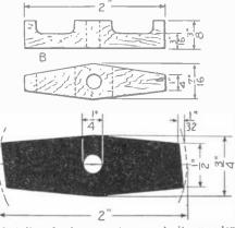
Details of the armature and its wooden clamps of the miniature motor. The lower drawing shows an armature lamination, This peculiar shape is required to carry out the unusual operation.
