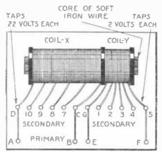
The illustration shows a transformer which combines the advantages of the auto-transformer, and the ordinary two-coil transformer. With why ten taps the voltage on the secondary can be varied from 2 to 120 volts in steps of two volts.
