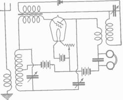
Fig. 2. Another method of reflexing using one tube and crystal detector. The primary is semi-aperiodic, the secondary is 60 turns tapped at the 30th turn. Both variable condensers are of .0005 mfd. capacity. method inasmuch as tests have shown this to be the most efficient. In the parallel connection it is necessary to insert a choke in the audio circuit, otherwise the secondary of the coupler would be short circuited due to
