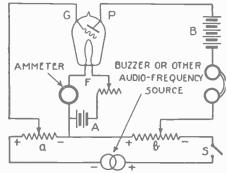
Fig. 2. The diagram represents the electrical circuit used for the determination of the coefficient of amplification. The ratio of the resistances b and a after having been adjusted to give minimum sound in the receivers, evaluates the amplifying qualities of the tube.
