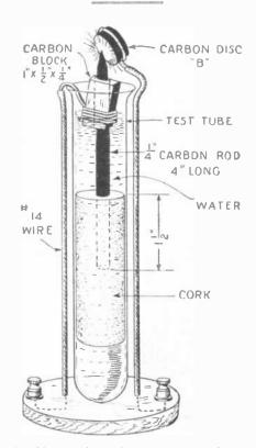
In this experimental arc-lamp a continuous feed of the lower carbon electrode is insured by the upward pressure of the water on the cork which carries the electrode in question.
