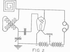
FIG 2 The same circuit shown in Fig. 1 using a op antenna. Note that the connection is loop uni-lateral
