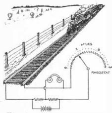
This Wheatstone bridge arrangement will enable you to determine the distance at which the approaching or receding train is located at any moment. A rheostat is adjusted until the sound in the receiver is at a minimum.
