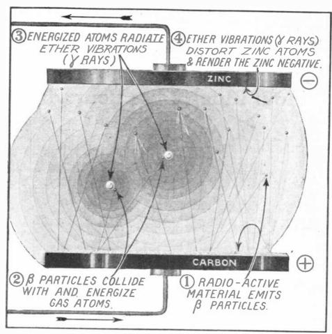
The electronic cell operating by the action of electrons emitted by radio-active substance placed on the carbon plate. Through ionization by collision with gas atoms ether vibrations are set up which charge the plates to opposite polarities. Mr. Kramer, the inventor of this cell, has constructed batteries of such cells with a potential of 25 volts.
