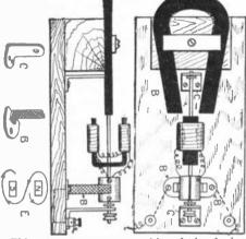
This electric motor capable of developing some useful power is designed after the form of one of the earliest electrical motors. Its field is a permanent horseshoe magnet. The winding of the armature coils is shown diagramatically at (E).
