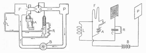
Fig. 1. The illustration shows a hydraulic system analogous in construction and operation to the electrical vacuum tube circuit. The flow of electrons in the electrical circuit is likened to the flow of water in the hydraulic circuit, and hydraulically actuated valves in the latter system correspond to the action of the grid and filament of the vacuum tube.
