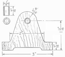
Detail of the bearings. The bearings proper are metal bushings inserted tightly fitting into holes in the top of the wooden frame.
