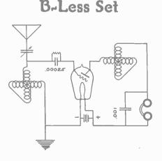
found that the set regenerated even better when the plate variometer was in tune with the grid. Using a Western Electric 216A tube, this circuit works very well on a six-volt A battery. With a DeForest DV3 it will work on two dry cells as the sole power supply (two flashlight cells, if you wish, make a very compact set). --Contributed by Powell Ross.
