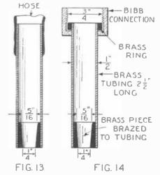
Nozzles, one for receiving a hose connection, the other for a bibb connection for driving the hydro-motor. They fit the hole in the upper part of the casing.
