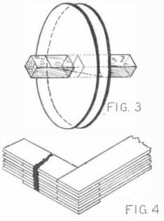
Fig. 3 illustrates the construction of a man-drel for the forming of the secondary coils. After the coil is wound, the mandrel is readily removed from the center. Fig. 4 shows the structure of the core laminations.
