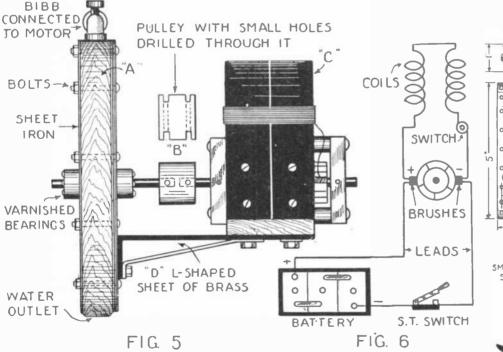
Fig. 5 shows the generator carried on a bracket attached to the side of the water motor. Fig. 6 gives the general layout or hook-up for charging a storage battery. Figs. 7 and 8 show the gongs drilled for the reception of the dippers and also the dippers in place.
