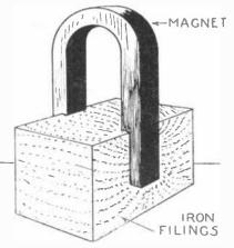
A neat paper weight for the experimenter, from flings sprinkled on the sides of the block are permanently fixed by the application of shellag or paraffine.
