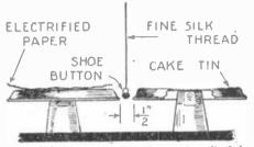
An addition to the experiment described in the January EXPERIMENTER. A pendulum is kept in oscillation by static discharges.
