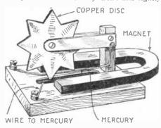
A simple form of the famous Barlow's wheel, Current flowing from the center to the periphery of the wheel reacts with the permanent magnet to produce rotation.
