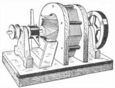
This perspective view of the minature electric motor shows effectively the construction of the commutator and armature.
