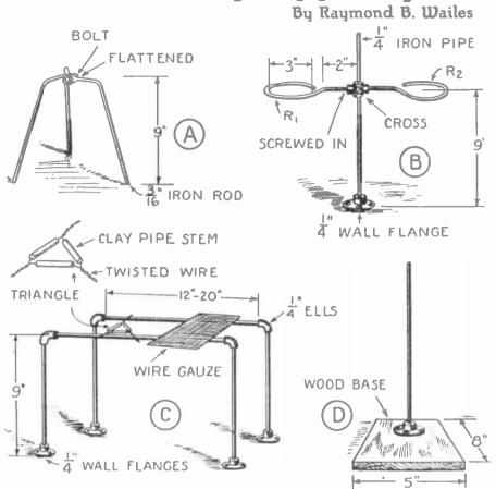
Various chemical apparatus made out of pipe fittings and pipe are shown above. Especially the use of the wall flange is to be noted, as this gives an exceedingly firm support and also makes an admirable foot for such pieces as do not require to be screwed down. The triangle is made of twisted wire and pieces of the stem of a clay pipe are strung upon it as shown, to avoid contact of a cruebble or other vessel placed on it with the iron. They also prevent the oxidation of the wire.
