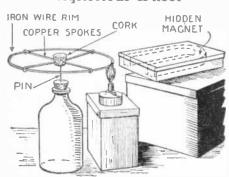
This mysterious rotating wheel made of iron and copper wire is actuated by the reaction between the hot and cold portions of the rim and the hidden magnet.
