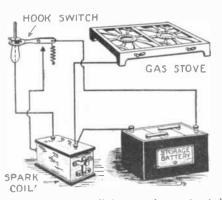
A handy gas-stove lighter can be constructed with the aid of a small spark coil and a stor-age battery. In lighting the gas is turned on and the electrode is brought near to or touched to the metal burner. A small spark ign.tes the gas.
