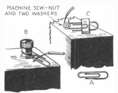
Many forms of terminals are adapted to rapid connection and disconnection by the use of the ordinary paper clip is illustrated above.
