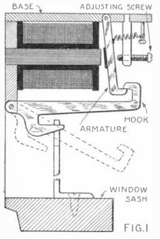
This electromagnetic release retains the window in open position until the magnet is energized. The armature then releases the hook and the window closes.
