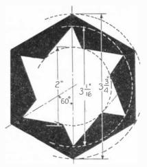
The stator of this 220-volt miniature motor is made up of soft iron laminations of the shape shown in black above.
