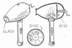
Pictures arranged on hand-rotated disc Fictures arranged on a hand-rotated disc illuminated by a pocket flashlight make this a very entertaining and novel toy. The pic-tures are observed through a small window. The toy is detachable from the flashlight. Patent No. 1,516,718 issued to C. I. Dailey, Jeffersonville, Ind.
