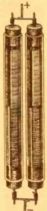
Trouvé moist cell, above. Elements of copper and zinc between which are several discs of blotting paper, half of which are wet with a solution of zinc sulphate and half with a solution of copper sulphate. When not in use, the discs are allowed to dry.
