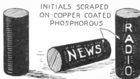
A method of preserving phosphorus in the air without any danger of spontaneous ignition. A very simple experiment and one of considerable interest.
