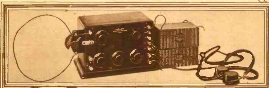
5. The oscillator below was designed to radiate short waves of from eight to about twenty meters length. To cover this range, replaceable inductances of one-, two- and six-turn coils are provided.
