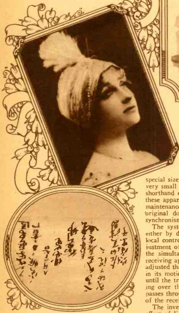
The two pictures above were transmitted by radio by the Belin method. The lower picture shows Chinese script which could not be transmitted by the ordinary telegraph systems.
