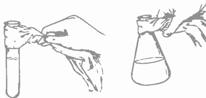
How to hold test tubes and small flasks with a towel or even with a folded wisp of paper. Such a wisp of paper is an excellent test tube holder.
