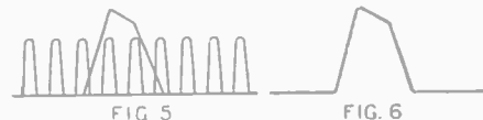
FIG. 5. Rectified signal and static waves received in circuit No. 1 of Fig. 2. FIG. 6. Rectified static waves received in circuit No. 2 of Fig. 2. This indicates that the rectified static waves in both circuits are identical.
