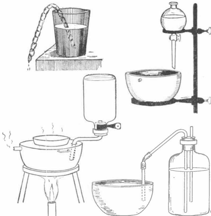
Various laboratory appliances are shown here. Above on the left is shown the capillary siphon which delivers water drop by drop, while on the right what is known as a separatory funnel is shown, which can be adjusted to do the same thing. Below these two are shown water supply systems which maintain an approximately constant level of water in a vessel from which water can be taken or evaporated.
