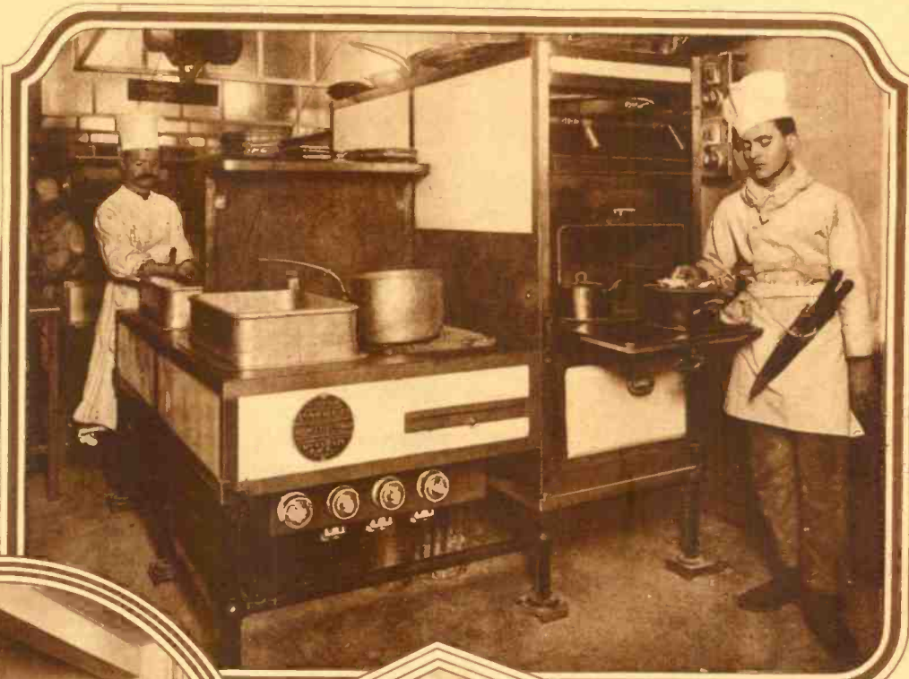
Right: Range for making sauces, with two heating elements and three-stage ovens. These and the other ranges are operated by electric heat.
