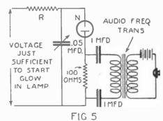
Another form of the "oscilloscope" is shown above. The secondary circuit of the audio frequency transformer is here coupled through a low resistance, to the neon tube oscillator.
