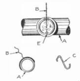
How the chimney damper is operated by the motion of the clock in order to turn on the draft before the occupant rises.
