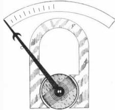
Fig. 2. A moving coil instrument. Here the pivoted core is in the opening of a coil of wire surrounding it, core, coil and index all moving together. The current goes through the coil.
