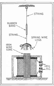
This curious toy spider is suspended over a hidden electro-magnet supplied with alternating current and will jump up and down in accordance with the frequency of the current. Its legs, made of steel springs, will go through humorously uncanny vibrations.
