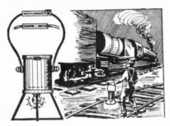
This lantern is provided with a large electrical battery lighting a small but powerful incandescent bulb. The novel feature of the invention is the use of the supporting arms as part of the electrical circuit of the lamp. The arms are threaded at the upper ends and screwed into an insulating handle. By turning this handle the operator can bring the ends of the arms together and thus close the circuit. circult.
