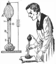
Instead of immersing the object to be plated, in the plating solution, the latter is applied by means of a sponge in the ingenious arrangement illustrated above. The solution is fed to the sponge through a glass tube in which an electrode connected to one terminal of the battery makes contact with the plating solution. The other terminal of the battery is connected to the object to be plated.
