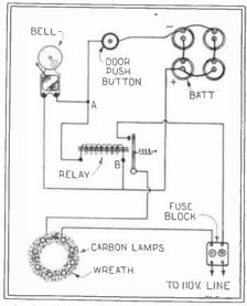
A cheerful welcome is extended to callers by this Christmas wreath mounted on the door and illuminated every time the door-bell is rung. A relay in the bell circuit closes the 110-volt lighting circuit through the lamps on the wreath.
