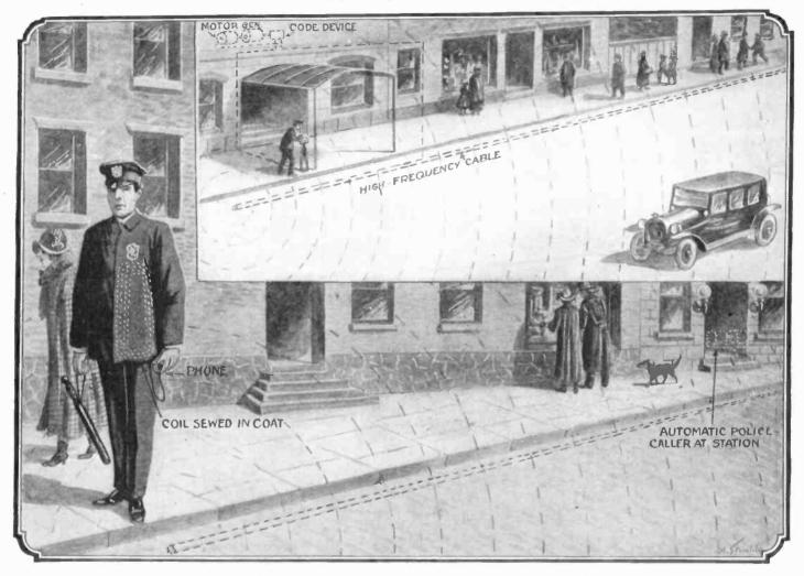
By means of an underground cable serving as a radiating antenna, signals can be communicated to walting chauseurs and policemen, who carry in car or on their person small coils which act as receiving aerials in connection with a small receiving set. This device eliminates the necessity for constant watching of electric signals, at present in use.
