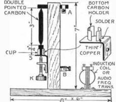
An induction coll or audio frequency transformer used in connection with the carbon rod microphone forms an excellent large amplitude microphone for experimental work.
