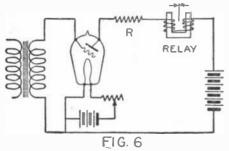
In recording radio messages through the action of an electro-magnetic relay, the introduction of a resistance R in series with the relay is necessary to accelerate the action of the latter.
