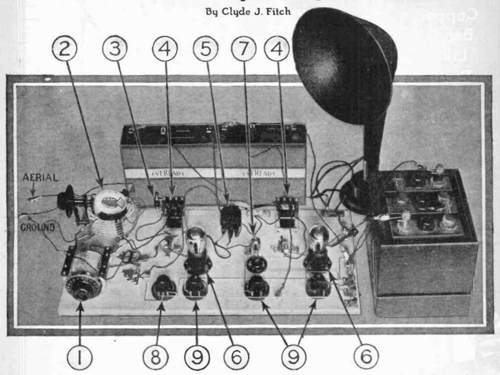
The two tube hook-up board with circuit No. 5 on the opposite page connected. The numbers designate the following instruments:
