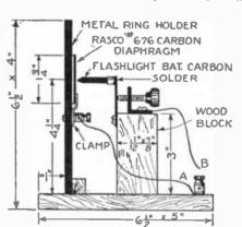
An interesting and novel variation of an old theme is shown in this illustration of an experimental microphone. A sharply pointed carbon rod in contact with a loosely supported carbon diaphragm assures a high degree of sensitivity.
