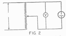
The illustration shows diagrammatically a circuit for the study of the behavior of the neon lamp under various potentials.
