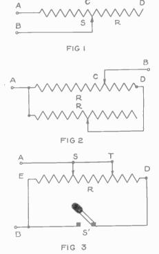
Fig. 3 represents a single resistance designed to accomplish the effects of the two rheostats in Fig. 2; an advance on that and on the single rheostat Fig. 1 used so much by experimenters.
