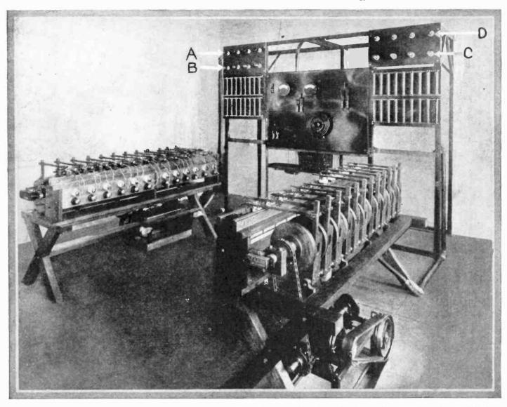
Apparatus for testing lamp switches, lamp sockets and the like. A number of such can be put on the apparatus and opened and shut in quick succession any desired number of times, to test their durability.
