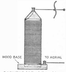
Constructional details of the moduloscope. This instrument is used as an ordinary Tesla coil except that it is excited by an undamped high frequency current. The voltage glow at the upper end of the coil indicates the degree of modulation when used in connection with a C.W. telephone transmitter.
