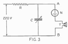
By varying the capacity of the condenser shunted across the neon tube in the circuit shown above, the frequency of pulsations of the current through the neon tube can be varied. The lower frequencies can be observed by periodic flashing of the neon lamp. The telephone receiver in the circuit enables the operator to listen to the pulsations.
