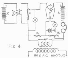
Hook-up showing how the amplification factor of a tube is measured directly by the dynamic method.
