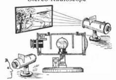
This apparatus combines in one unit the means for stereopticon projection and for the close examination of pictures. An adjustable magnifying device provided with an eye-piece enables the operator to make a close examination of the pictures, which, when placed in the other slot indicated in the diagram, can be projected through a large lens on a screen. Patent 1.504,989 issued to B. L. Slitzer, New York, N. Y.
