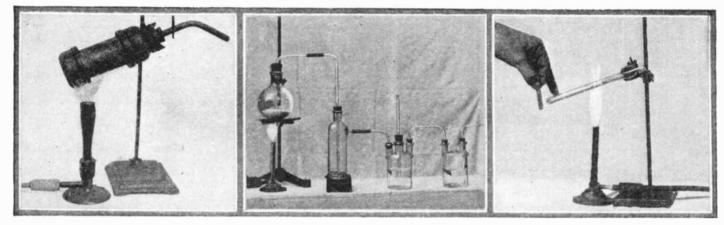
The evolution of gases, 1, by destructive distillation on the large and small scale, 2, by double decomposition and, 3, by the decomposition of a chemical, by the simple application of heat, are shown in experimental guise above.
