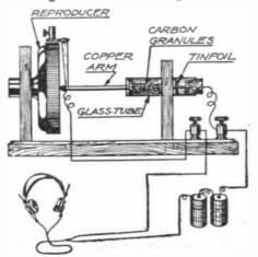
end of the copper arm enters the glass tube but does not bind in it. Put some tinfoil in the glass tube close to one end; fasten a wire to the tinfoil and then to one of the binding posts. Put a few pieces of carbon in between the copper arm and the tinfoil, and connect a wire to reproducer
