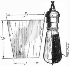
A compact reflector is obtained by this ingenious arrangement of tinfoil attached to one side of the glass bulb of an incandescent lamp.
