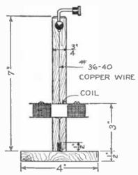
The galvanometer here shown in section is within reach of every experimenter. It is of the moving coil type with wire suspension, one absolute requirement being a strong horseshoe magnet with broad poles.
