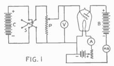
Hook-up showing how the characteristic curve of a vacuum tube is measured. The curves shown in Figs. 2 and 3 were obtained with these connections.
