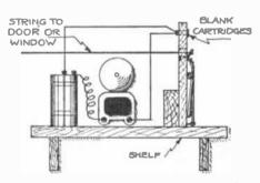
The general hook-up and string connections for the rat-trap burglar alarm. Note the cartriages,
