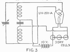
An oscillator employing a type 201-A tube operated with three dry cells for the filament and ten volts for the plate.
