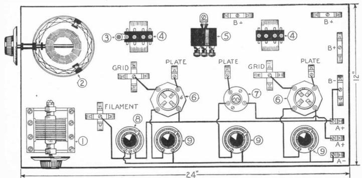
Details of the two tube hook-up board showing the location of the instruments and binding posts. The connections of the filament circuit are also clearly shown.
