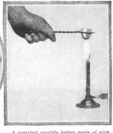
A practical crucible holder made of wire is shown as a substitute for the regular chemist's tongs.
