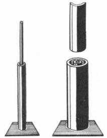
The moulds illustrated above enable the experimenter to make rods or hollow cylinders of carbon. The battery carbons so formed must be dried and baked after removal from the mould.
