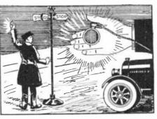
As shown in the illustration this electric As shown in the illustration this electric signal lamp contains a small incandescent lamp in a compact case which lamp is connected to a flashlight battery carried in the pocket. The circuit can be made or broken by means of the push-button operated by the thumb, the entire case being attached to the fingers by means of a small strap.
