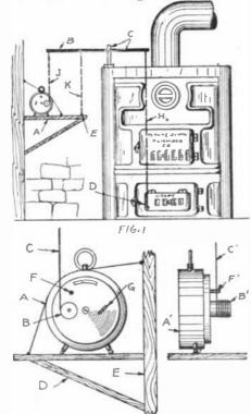
A perfected arrangement for opening the dampers of a furnace by an alarm clock. This is shown as operating a hot air furnace, but of course can be applied to other types of
