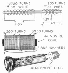
A night light made out of a flashlight case which contains within Itself the transformer. It is supposed to be adapted for use on a 110
