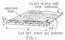
To make the mysterious glass strip that will yield both positive and negative charges, cut a strip such as indicated in the figure from a plate of glass, one side of which is ground.
