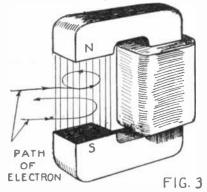
Charged particles such as electrons moving in a magnetic field are considered to follow a circular path. In fact, in a very strong magnetic field an electron moving with a comparatively small velocity may be forced to move in a circle without leaving the field.
