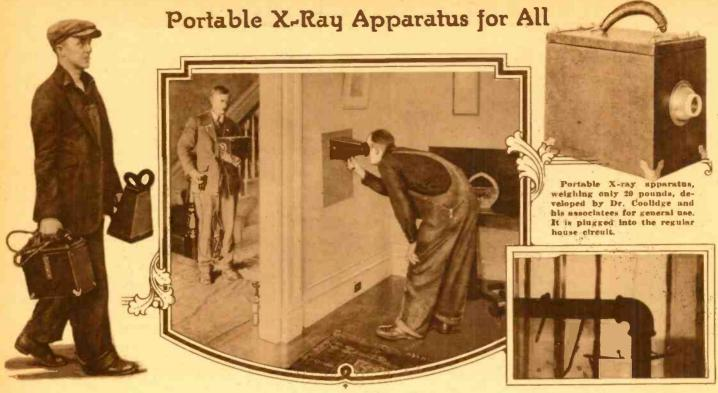
A plumber carrying the outfit to his work has in one hand a fluoroscope and he uses it for looking for pipes behind the plaster and woodwork of a house.
