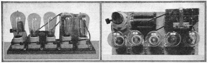
Left, front view of the B battery supply unit showing the five lamps used as resistances. The 50-watt lamp at the left protects the apparatus from accidental short circuits and tube burnouts.
