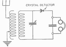
Diagram of the crystal receiver. The crystal detector indicated is merely a metal wire in contact with the metal detector holder.
