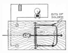
Let your rat-trap protect you against burglars. An ingenius suggestion is indicated above; when the trap is sprung it not only closes an alarm circuit, but discharges two blank cartridges.
