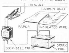
A curious electro-static experiment is illustrated above. The secondary lead from a Ford spark coil is brought near a small pile of carbon dust on a piece of paper. As the primary circuit is closed the electro-static field set up by the secondary potential will cause the carbon particles to assume positions in wave-like circles.
