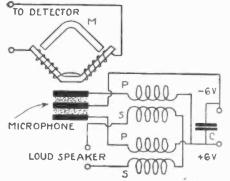
Connections of the amplifier used in the Crystovox. Note that two chambers of carbon granules are used.
