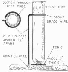
A simple test tube holder. As shown it holds a single test tube, but by using a long strip of wood for the base and a number of wires it can be made to accommodate any number.
