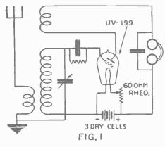
Hook-up showing how a UV-199 tube may be operated without a "B" battery. In this case the drop across the rheostat is sufficient to produce a current through the headset.
