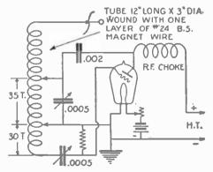
An oscillatory circuit suitable for exciting the Moduloscope coil. A Tesla effect is produced at the upper end of the coil causing the small wire to spin around. The ordinary short wave C.W. transmitter may be used for making these interesting experiments.
