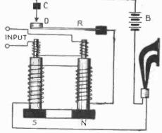
An earty form of Brown relay. A regenerative effect is produced by the larger winding in the microphone circuit that encircles the magnetic core
