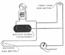
An electric bell operating through a transformer and made to give two distinctive sounds by having two circuits of different resistances through which it is rung by two push-butttons.
