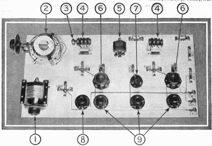
Plan view of the hook-up board showing the instruments mounted in place. The instruments shown are as follows: 1. Condenser; 2. Low loss tuner; 3. Crystal detector; 4. Audio transformer; 5. Radio transformer; 6. Socket; 7. Diode socket; 8. Potentiometer; 9. Rheostat.
