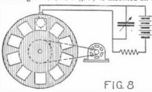
The diagram illustrates the action of the "stroboscope." The periodic flashing of the neon lamp is set in synchronism with the rotation of the large disc carrying near its periphery a series of pictures depicting the successive stages of some action. The resulting effect will be an illusion of continuous action.
