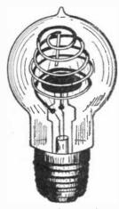
A common type of neon lamp is shown above. It consists essentially of two metallic electrodes located close to each other in a neon filled tube. The application of about 150 volts to the terminals of this lamp will cause the negative electrode to glow.
