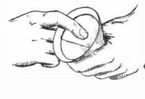
Folding a smooth filter paper. There are three ways of doing this, all of which are described in the article. If the funnel is exactly a 60 degree funnel, so-called, a paper folded as described will fit it exactly. But as this is not always the case, the last fold of the paper can be given inside the funnel, by a sort of rolling motion of the index finger moving toward the place where the fold will come.
