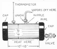
The dimensions of a simple retort for making coal gas upon a larger scale, as described in the article.
