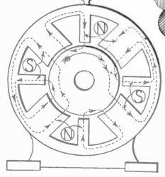
practically balance at all currents. The strength of these poles is therefore automatically regulated, which tends to provide a rigid magnetic field at all loads and speeds for which the machine is designed. The position of the neutral plane of minimum induction will remain practically constant.
