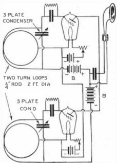
A form of electric balance is illustrated above. The beat note produced by the interaction of two circuits oscillating at different frequencies is altered when conducting substances are brought near one of the two loops shown in the circuit. The apparatus may thus serve as a detector of under-ground metals.
