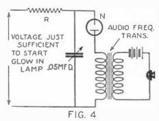
The diagram shows the connections for the neon tube "oscilloscope". By means of this device the modulations of sound impressed upon the microphone are "rendered visible" by the varying intensities of the glow of the neon tube.
