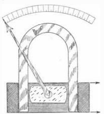
Fig. 1. Diagram of the construction of a moving armature instrument. The coll acts at right angles to the field of the magnet and moves the armature carrying the index.
