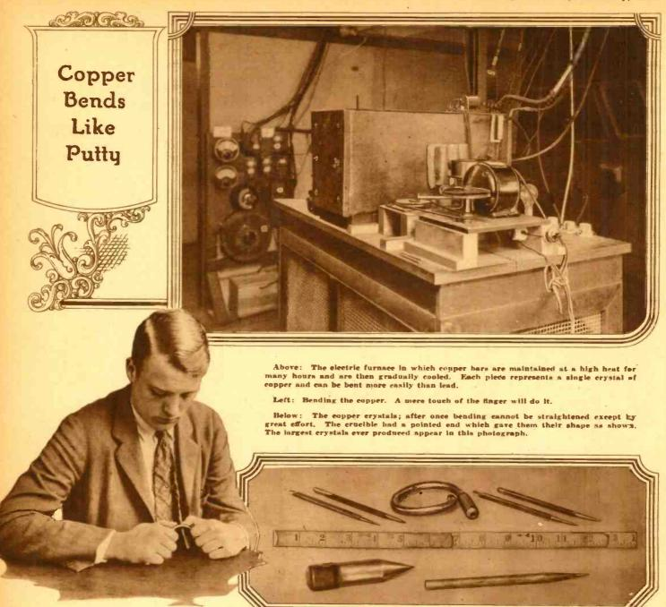
OPPER bars that can be bent double with one finger, but which require strength to straighten again, are expected to lead to a greater understanding of the properties of metals. The bars, which are really single crystals of pure copper, were produced in the Research Laboratory of the General Electric Company at Schnectady, N. Y., and have been subjected to many kinds of examinations, with the revelation of numerous unexpected facts.
