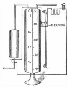
The simple but effective device shown above will do much to reduce the gas bill in connection with hot water furnaces. An alarm bell actuated by a thermostat will ring when hot water of the required temperature has reached the level to which the rheostat is adjusted; the latter can be shifted along the length of the furnace,
