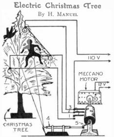
An animated Christmas tree with flashing electric lights can readily be constructed with apparatus assembled in the experimenter's laboratory.
