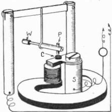
The Tauleigne amplifier. This Instrument has met with commercial success in France. A microphonic contact is made between the two electrodes C and P.
