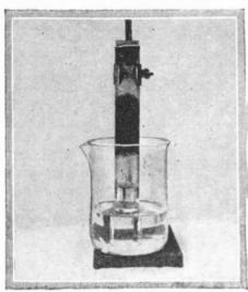
The combination of oxygen with iron, the experimental demonstration of the rusting of the metal.
