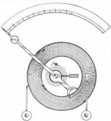
Fig. 3. An eccentric vane instrument in which a hairspring brings the index back to zero and holds it there. When current passes through a coil, an eccentrically pivoted armature is attracted and moves the index.
