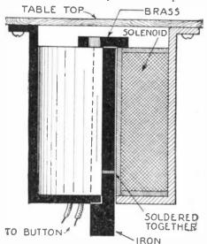
The amateur magician will find the table knocker illustrated above an effective device in mystifying the credulous and baffling the skeptical members of his audience. The device is merely a solenoid and plunger mounted underneath the table top and through an invisible wiring supplied with current from a dry cell. The knocker is actuated by means of a push button carried by the demonstrator.
