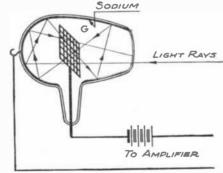
Diagram of a sodium photo-electric vacuum tube; a surface of metallic sodium emits elec-trons when light falls upon it, and these carrying their charges form a virtual conductor.
