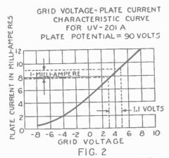
A characteristic curve of a 201-A tube showing the relation of the plate current with various grid voltages.
