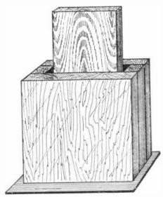
This simple form made of pieces of board affords a very satisfactory mould for tamping the coke and graphite mixture to be used for battery carbons. The form shown above is used for making carbon plates. Some gluecose syrup or other binder is mixed with the pulverized material.
