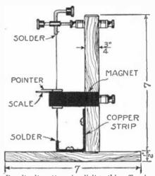
Despite its utter simplicity, this efficacious galvanometer can be finely adjusted with respect to coil position and the tension in the suspension wire, by means of the adjustment screws at the top of the apparatus.
