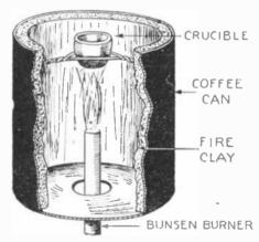
A coffee can lined with fire clay encloses the flame of a Bonsen burner so as to constitute a species of furnace; a very good home-made appliance for laboratory use,
