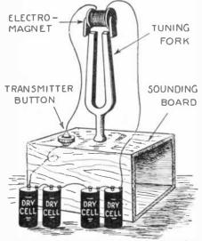
Complete synchronism between the vibrations of the tuning fork and the interruption of the current through the electromagnet is accomplished by the introduction of a microphone in the electrical circuit.
