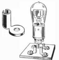
Vacuum tube per lugs mounted on a hard rubber base. The low capacity and losses make it ideal for abort wave experiments.
