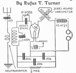
A super-regenerative circuit of a Flewelling type. This receiver is claimed by the writer to give results equaling those obtained from the ordinary detector and two stage amplifier. in using the Flewelling receiver would be relieved if transformers, fussy crystal detector, etc., could be dispensed with and the desired results are obtained more readily.
