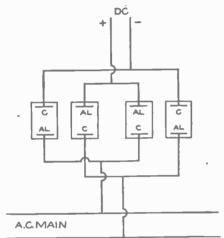
The diagram shows a four-cell electrolytic rectifier provided with aluminum and carbon electrodes. While such rectifiers have been constructed for heavier currents, the experimenter will find its operation most efficient on currents of less than one ampere.
