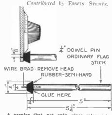
A vernier that not only gives micrometer adjustment but eliminates body capacity ef-fects is easily made with a dowel pin and rub-
