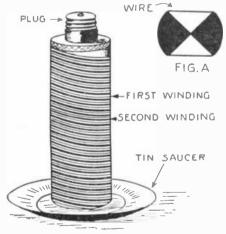
A diabolic device for the electrocution of the house-fly; as he alights on it he bridges a gap and closes a circuit.
