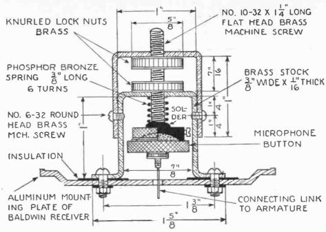
Details of an amplifier employing a transmitter button that may be attached directly to the front mounting plate of a standard type C Baldwin receiver.
