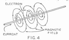
It is well known that a current passing through a conductor sets up a magnetic field as shown above. An electron emitted by a heated conductor will, if the field is strong enough, be constrained to move in a circular path and be forced to return into the conductor.
