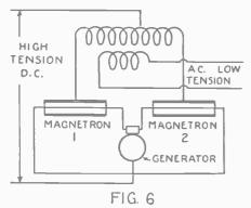
This diagrammtic view of the electronic converter shows the disposition of two Magnetron tubes in connection with a specially designed generator supplying the filament current. This unit will receive high tension D.C. and supply low tension A.C. of any frequency or receiving low tension alternating current it will supply high potential D.C. high potential D.C.
