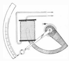
Fig. 4. The solenoid instrument. Here a solenoid is provided with a curved core, which is attracted to a greater or less extent by the current in general proportion to its strength. A very simple and useful instrument.
