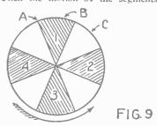
A rotating disc such as that shown above observed by the light of the neon tube oscillator gives rise to an illusory apparent motion which may differ in speed and even in direction from the actual rotation of the disc.
