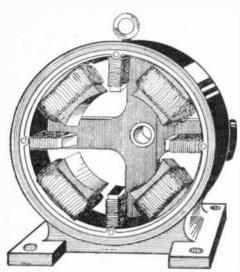
In order to improve commutation and prevent the necessity of shifting the position of the brushes for changes in speed or load of dynamos and motors, small auxiliary poles, called "inter-poles," are sometimes provided in addition to the regular poles of the machine. These interpoles, as the name implies, are placed between the main poles of the field as shown in Fig. 1.
