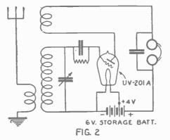
Circuit showing a type 201-A tube operated with four voits on the filament and two on the plate. Dry cells may be used.
