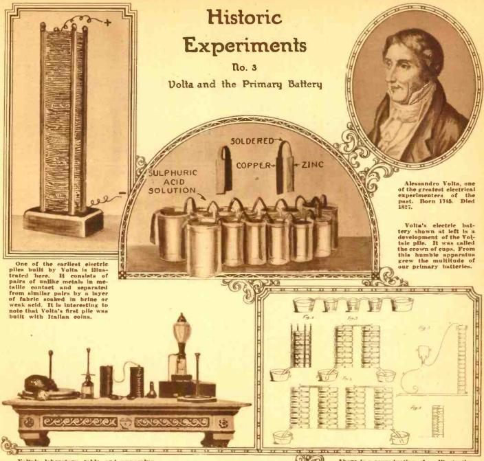
Volta's laboratory table and apparatus has been preserved in the Instituto Lombar-do di Scienze, in Milan. Note the electro-phorus at either side and the Voltaic piles in the center.
