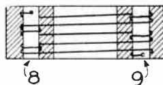
Fig. 14. The thermic wires are here supported by little cylinders of insulating material.
