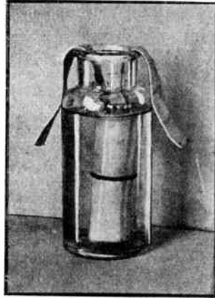
Complete Planté storage battery set up; one which can be made by the amateur and which will give excellent results for the lighter class of work.
