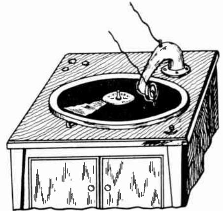
The phonograph disc, reproducer and microphone, showing the microphone and the electric connections to the microphone.
