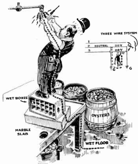
An accident which might have been a very serious one, due to the fact that the electrician stood upon a wet support. A very bad shock was received.
