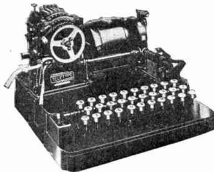
The combined receiving and transmitting instruments; the keyboard is used for sending and is copied from the standard typewriter keyboard.
