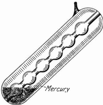
An astral tube, producing a very pretty Geissler tube effect, when shaken.
