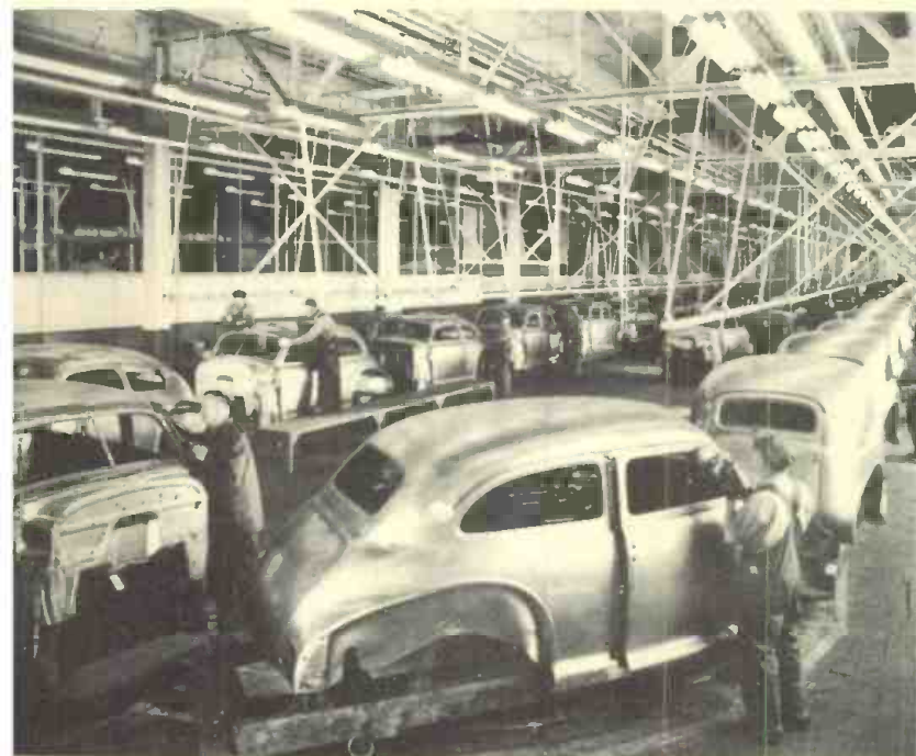
Here the bodies at Fisher Plant Number Two get a final metal finishing.
