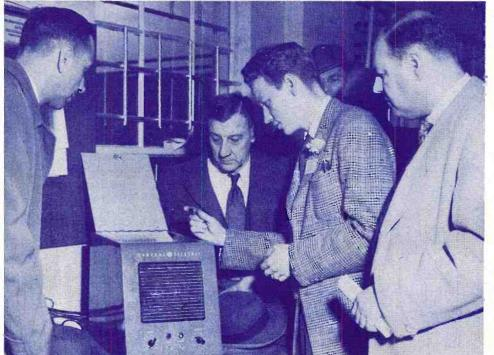
Close-up of GE high frequency FM emergency communications receiver used to pick up messages from transmitter in auto 50 miles away.
