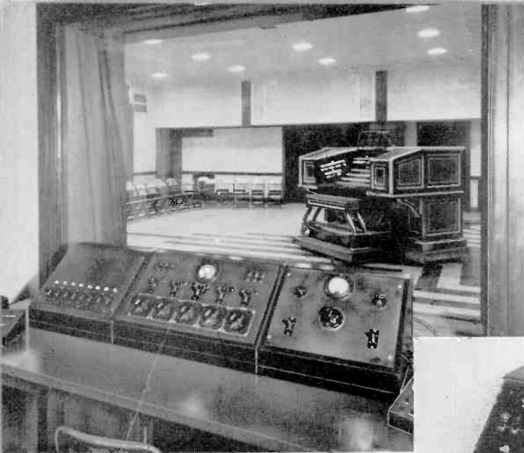
Studio control console, at left, at which the operator regulates and controls the output from the one of more microphones in use in the studio.
