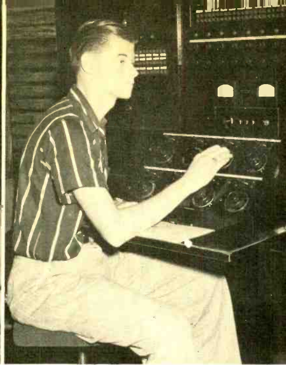
John Heslip is "riding gain" (Regulating the volume and mixing the sound impulses from each microphone) on a studio program. Intensity of the sound must be kept within rigid limits.
