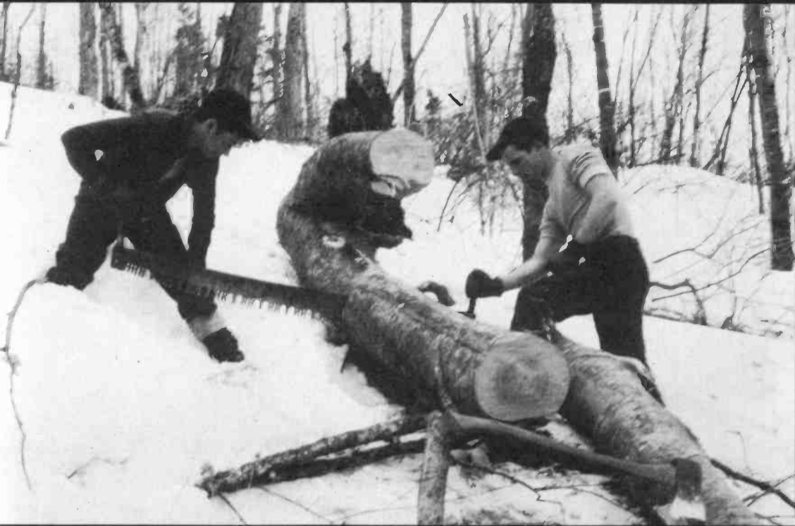
Backaches from the crosscut saw are now eliminated by power-driven chain saws
