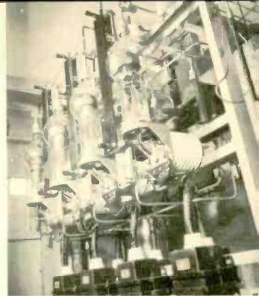
A few of the tubes necessary for sending out a 50,000 watt signal.
