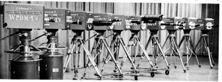
WFBM technicians constructed these ten cameras for use on studio and remote telecasts. These special cameras were built under the supervision of chief engineer, Harold Holland. WFBM-TV is believed to be the only television station in the country who made its own cameras.
