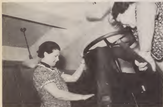
With this heavy cutting machine, Mrs. Katherine Mortlock, left, and Miss Valeria Sparks of the bindery can slice a stack of paper four inches high with a twist of the hand.
