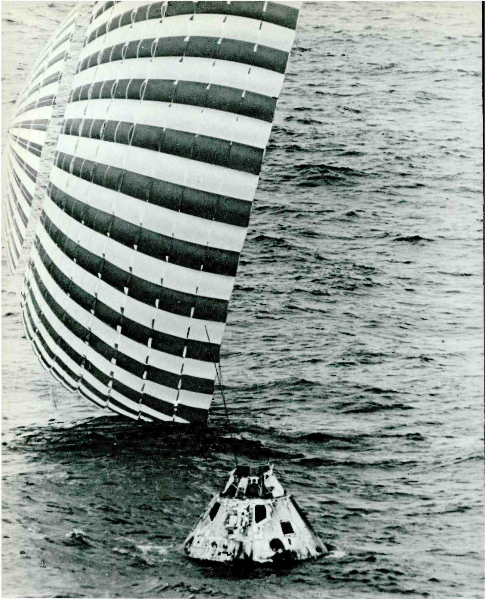
The Apollo 4 spaceship under its 83-foot-diameter parachute splashes onto the Pacific after its 9,000-mile unmanned space journey in November. It reached a peak altitude of over 11,000 miles in its 8½-hour flight.
