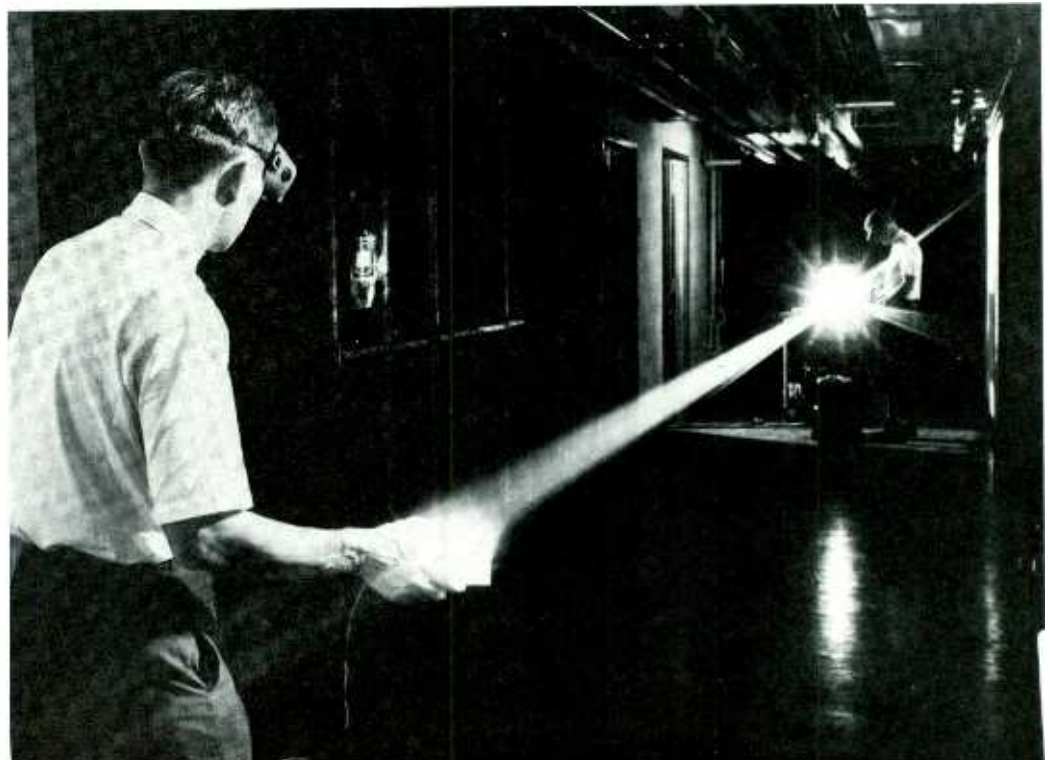
At RCA Laboratories in Princeton, New Jersey, scientists measure the characteristics of a 10-watt argon laser. The tightly controlled non-widening beam of light will be used by NASA in earth-to-space tracking and communications.
