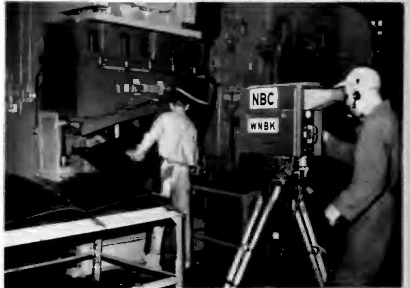
WNBK camera catches the huge presses of the Chevrolet plant forming hoods and fenders for automobiles.
