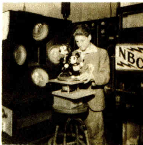
ABOVE: In the late Twenties, Felix the Cat and Mickey Mouse whirled for hours on a phonograph turntable in front of television "eyes," while engineers in the field made reception tests.
