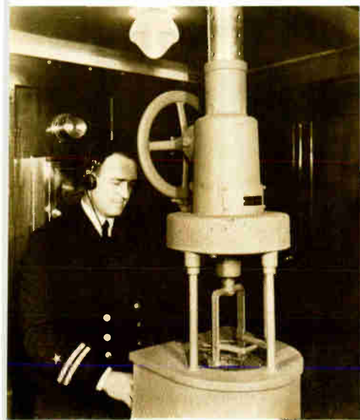
ABOVE: An RCA direction-finder installed in the chart room of an ocean liner spots the location from which radio signals originate.
