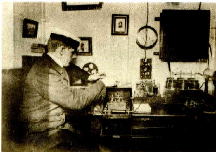
ABOVE: Early shipboard radio apparatus, as installed on the SS Minnehaha in 1904, featured a coherer with tape recorder and a spark-coil transmitter — a marked contrast with the modern, compact marine apparatus which utilizes electron tubes and establishes communication with land from any latitude-longitude on the Seven Seas.
