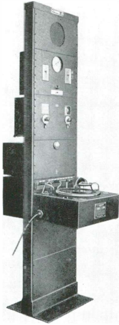
The control panel, through which the program is relayed to the various loudspeakers throughout the building.
