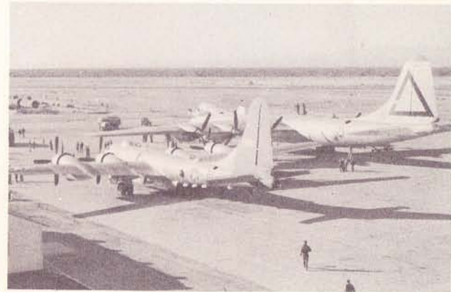
Lined up on the runway at Davis-Monthan are (left) a B-29, and beside it the newer, Very Heavy B-36. Many training and experimental flights-such as the recent non-stop around-the world flight- either originate at, or use equipment and personnel from Tucson's Davis-Monthan Field.
