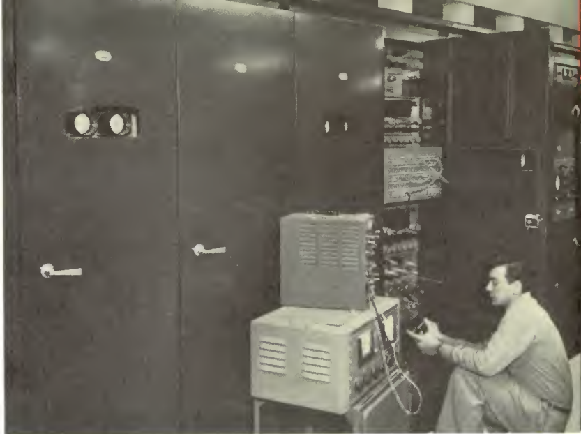
MORT ZIMMERMAN , left, KBTv transmitter maintenance engineer, is shown making adjustments on one of the many regulated power supplies for the picture distribution system in the transmitter room.
