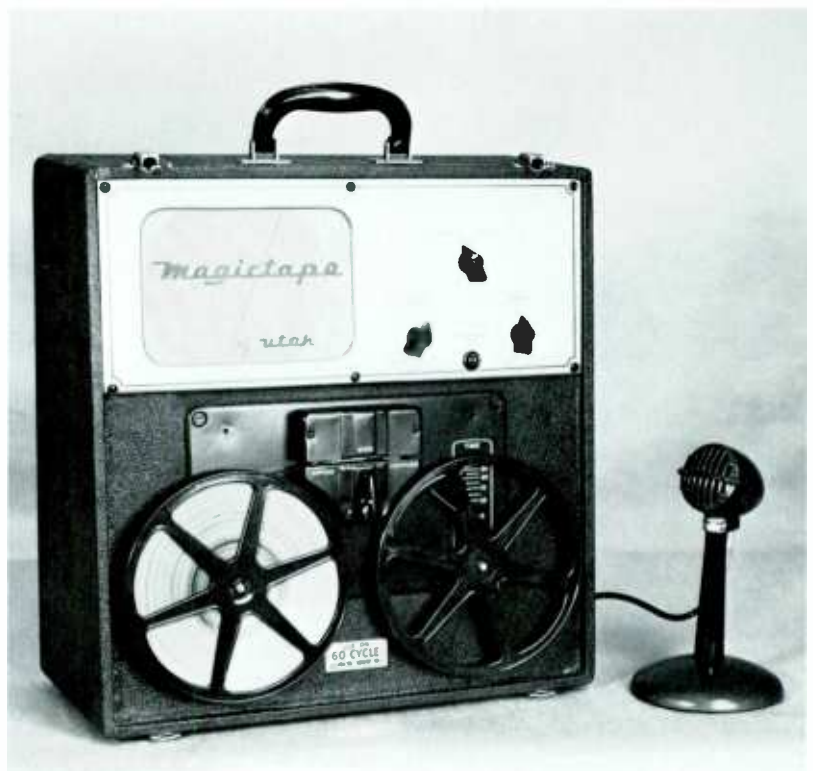
An early portable tape recorder, ca. 1947, threaded with a reel of paper-based recording tape. (VPL no. 28002)
