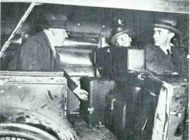
(LEFT) The Tribune station was not the first in Chicago, but it always played a vital role in giving leadership to its community. The first radio police car was devised by Carl Meyers, left, then chief engineer, now vice president of WGN, who built and installed a 7-tube set and small horn speaker here being tested by police in March 1929. Station broke into programs with police bulletins. (WGN)
