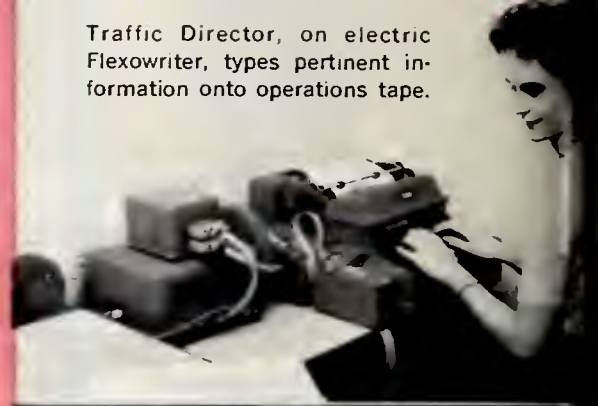
Punched tape is fed into “tape readers” which first stores information in master control data storage and processing area, and then actuates electronically timed and coded equipment into any switching operation desired.
