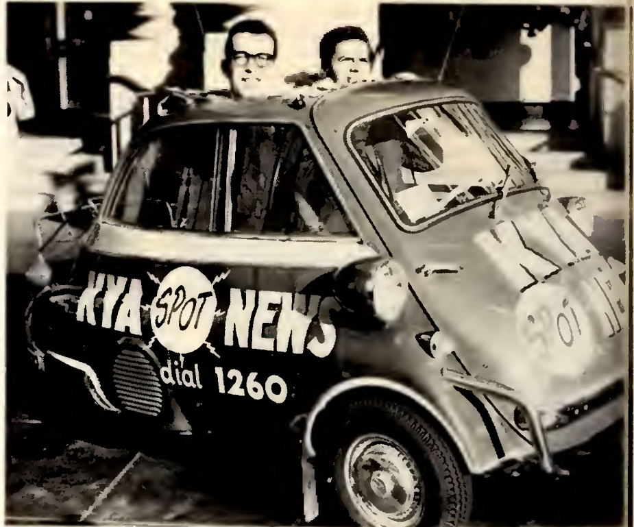
Roving Sputnik is used by KYA, San Francisco, newscasters to get spot news fast. Car is short-wave controlled and completely fitted with custom-designed broadcast setup for direct voice contact with station
