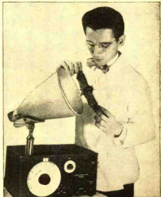
Bat, held before supersonic sound detector, is found to "broadcast" his own "beam".
