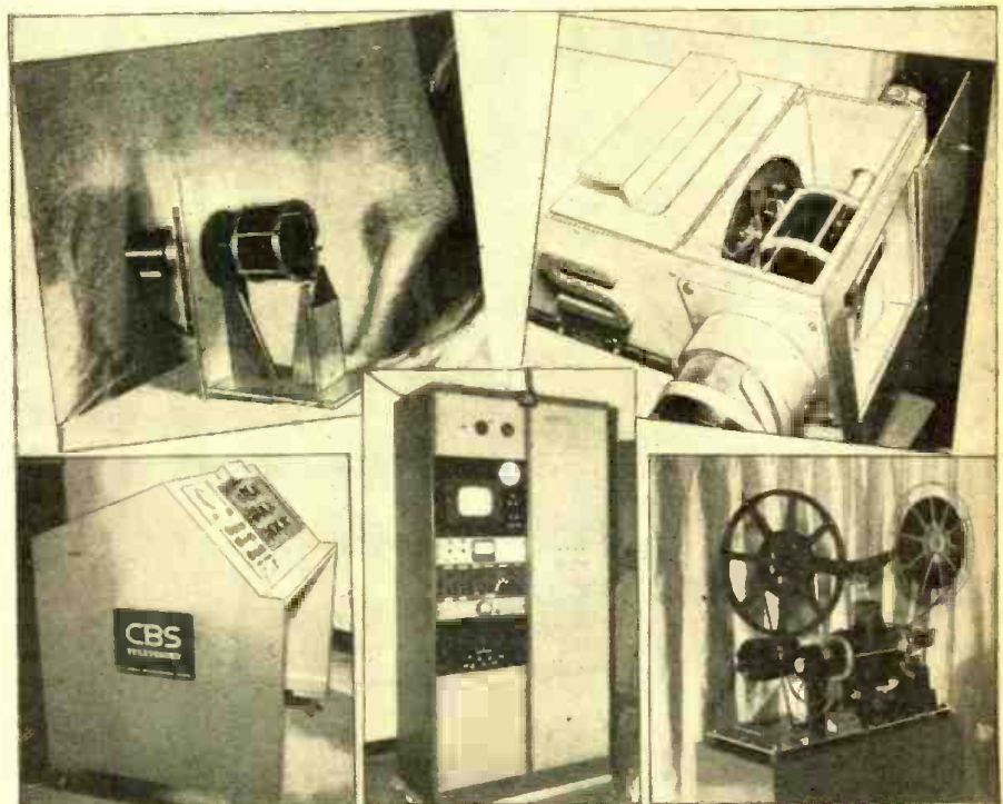
Upper left—the color filter drum which forms the heart of the CBS television scanner. Upper right—the drum in position around the orthicon. Lower left—control bench. Center—the amplifier rack, with CR tube for monitoring programs. Lower right—the film scanner for color television. Note: The receiver looks just like any black and white receiver from the outside, but inside there is a color filter wheel about twice the diameter of the viewing screen. This was described in a previous issue of RADIO & TELEVISION.
