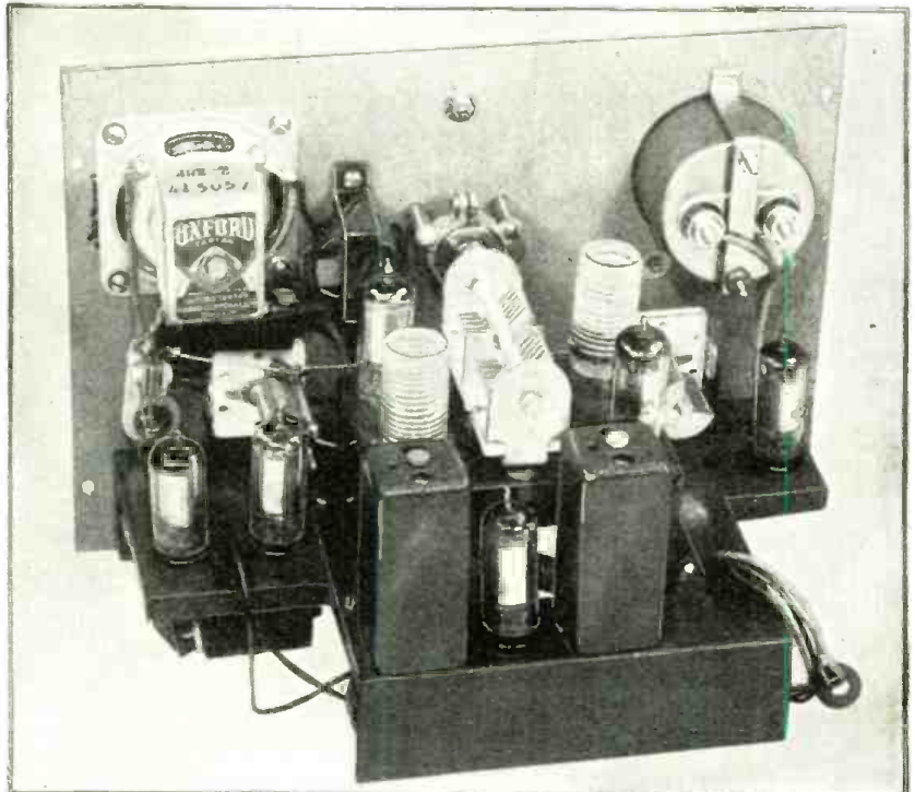
Rear view of the custom-built receiver, skillfully put together by its designer, Mr. McEntee—batteries not shown. Note loudspeaker at left and "tuning meter" at right.
