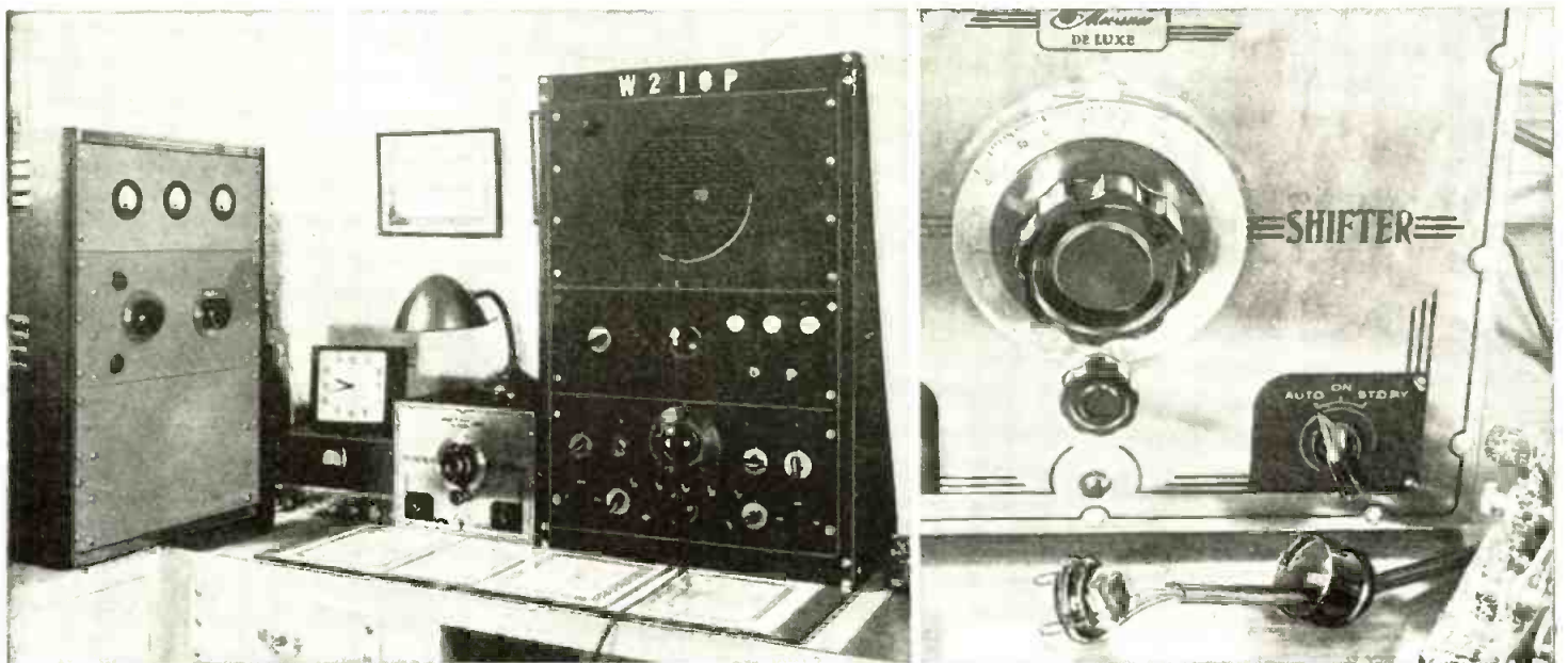
Left—The Contest Special "at home". Note the controls mounted in the rack with the receiver. The simplicity and beauty of the rig is apparent. ECO on one hand; "break-in" keying; the perfect set-up for good operating. Right—The ECO connector as explained in the text. Ordinary mike cable is used for the line, and a 5-prong plug for the container.
