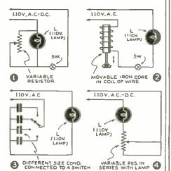
If you have a number of condensers of different capacity lying about, several of these may be connected to a switch as shown at Fig. 3; the lamp will light the brightest on the large size condensers, and dimmer on the smaller capacity condensers. One of the usual ways of dimming a lamp is to connect a variable resistance in series with it as shown in Fig. 4.
