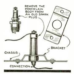
center of the plug. If space permits the mounting bracket may be installed underneath the chassis.-Richard Kroaman.
