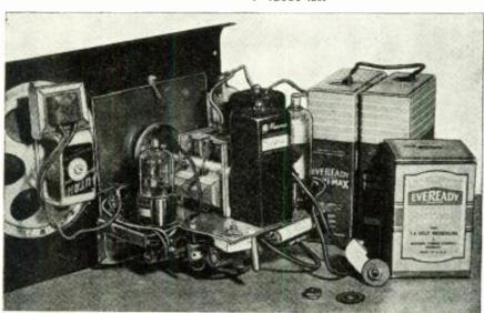
Here is a view showing all the parts, including the batteries, for building the portable 3-tube receiver, which does the work of 6 tubes.
