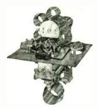
the plate coil to the respective stators. Further elimination of leads is accomplished by a pair of special brackets (type "BWZ") which mount two type "ZS-7-SS" "Trim-air" neutralizer condensers on diagonally opposite sides of the respective MT-100-GD stators, the transmitting tubes being arranged on diagonally opposite sides of the tank tuning condenser.
