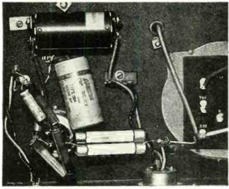
Closeup of Strobotron socket, showing resistor network.
