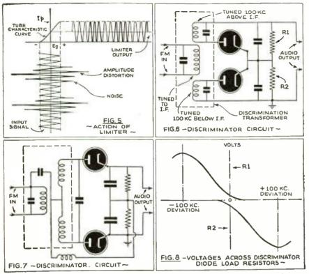
The action of the "limiter" is shown in Fig. 5. Typical "discriminator" circuits are shown at Figs. 6 and 7, and Fig. 8 shows the voltages across discriminator network.
