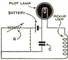
energy will increase its brilliance from dull red to dazzling white. The 70% of the energy is supplied by a small battery and variable resistor in series with the bulb and coil as shown in the diagram. Resistor R is adjusted until the bulb glows dull red. Condenser C may be any small condenser which is available. The pickup coil is now loosely coupled to the transmitter circuit. If a two volt .06 amp. pilot bulb is used, no
