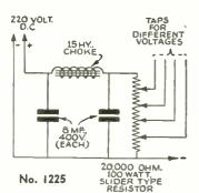
Please publish a diagram of a well filtered power-supply to operate on a 220 volt D.Cpower line.—P. E. Saldana, Palo, Leyte, P. I.
