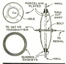
a good steel bit not over ¼ inch in diameter you can bore a neat hole. Be sure to keep the nail directly under the center of the plate where you are drilling.—Alton Larbenteur.
