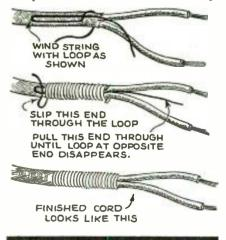
ping as possible. The cord will be firmly secured, and no knots or loose ends will remain.—Steve Liska.
