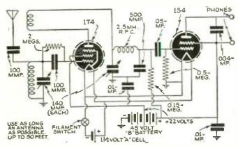
A 2-Tube Receiver for the experimenter. (No. 1227)
