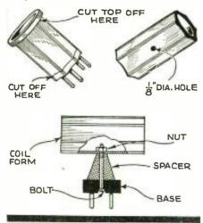
the two parts together using the upper half of a "pee-wee" feed through insulator as a spacer. The coil must be taken apart before the wire can be wound on it and when this is done one-half inch should be left between the two windings to accommodate the top of the spacer. This type of coil is very convenient in many applications and will not cost much more than 25 cents.—E. J. Rohrig.
