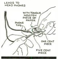
paper. This paper must be thoroughly moistened with saliva, which serves as electrolyte in the tiny battery. Touch one phone tip to the nickel and start tapping the penny with the other. If the phones are in working condition a faint click will be heard when the penny is tapped.—James Haluszczak.
