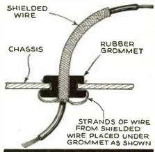
nection but also holds the wire in place and makes a neat end on the shield.-Oleg
