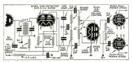
This interesting circuit was supplied by Harvey Gernsback, and shows the hook-up for an infinite-impedance second detector in a superhet receiver. Note that this circuit permits the second detector to feed the push-pull audio frequency amplifier stage, without the use of a transformer.
