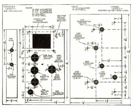
Layout details for the panel and the chassis of the receiver are given above.
