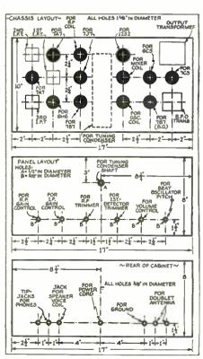
Above---Chassis and front panel drilling dimensions.
