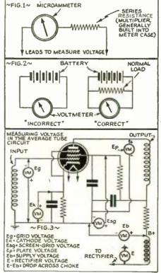
How and where to make voltage tests.
