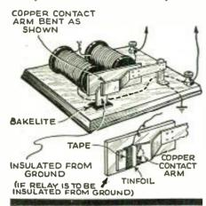
of the 10c store variety. The circuit of the buzzer is changed, the interrupter being disconnected from the magnet circuit. The magnet is connected directly as the primary and when energized attracts the rebent contact, causing it to close the secondary circuit. If necessary the relay may be rebuilt to insulate the contact arm bracket from the base.—Harry Greenberg, W2MSQ.
