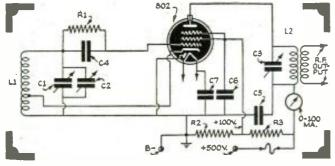
Electron-coupled oscillator for transmitter. No. 1210.
