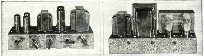
readily be overcome by means of a decoupling network but since this necessarily meant a reduction in gain, another method was used instead. It was found that increasing the capacity of the final filter condenser (C) from 8 mf. to 24 mf. completely eliminated all speech amplifier oscillation without the necessity of adding decoupling networks to the circuit.
