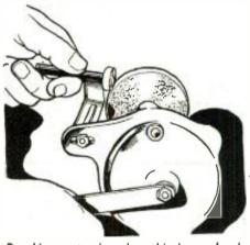
Roughing out glass lens blank on handoperated grinding wheel.
