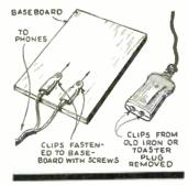
posts. However, I had some old plugs of the type used for electric irons and toasters. I removed the clips from these plugs and screwed them to the board, where they worked fine as phone jacks.—Dayton Baldwin, Jr.
