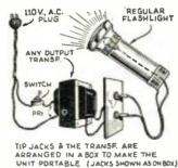
former, as shown in the accompanying sketch, as power for the flashlight used to inspect receivers in my service shop. Any output transformer will provide the low voltage high current necessary for flashlight bulb operation or, if one prefers, a filament transformer can be used, in which event standard pilot light bulbs can be operated in the flashlight at their normal brilliancy. And it's always ready when needed.—.4. Morino.
