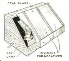
Construction of Comparator Box; standard negatives go in end frames, with new negative between them.
