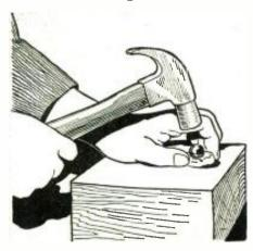
Ball bearing hammered into lead sheet makes grinding lap.
