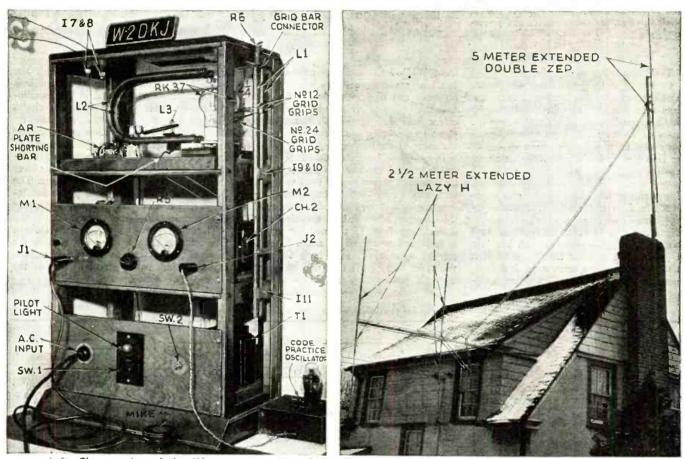
Left-Close-up view of the 21/2 meter transmitter. Right-The antennas used at Station W2DKJ for 21/2 meter operation.
