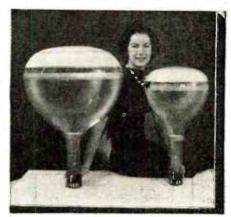
sistence screen, which is said to make it possible to use lower frame frequencies without flicker. The DuMont circuit is also unique in that the number of frames per second and the number of lines per frame can be varied from the transmitter. The DuMont tubes are also equipped with an exclusive intensifier feature said to produce brighter images without increasing anode voltages.
