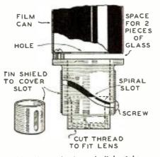
How focus slot is made light-tight.
