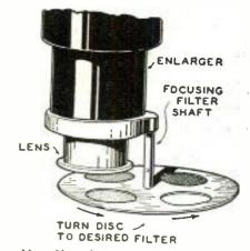
How filter disc mounts on enlarger.
