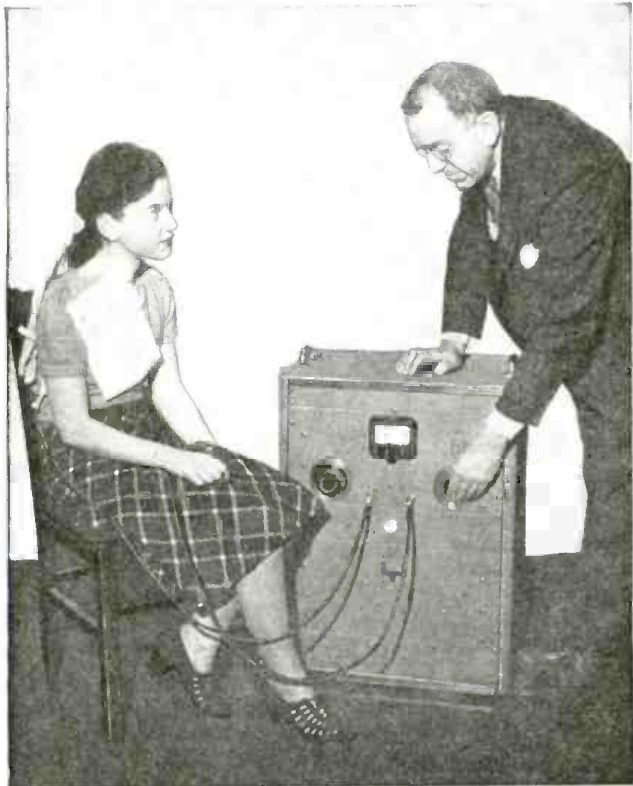
"Doc" Secor is here giving a treatment to a "patient." The electrodes shown are encased in washable cloth bags in order to absorb moisture. The left-hand knob controls the power output or "tuning," the right-hand knob is the 0-30 minute time twitch.
